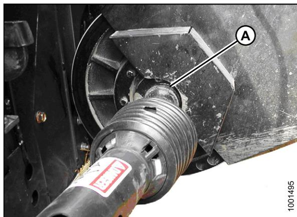
Figure 5.110: Disconnect driveshaft
