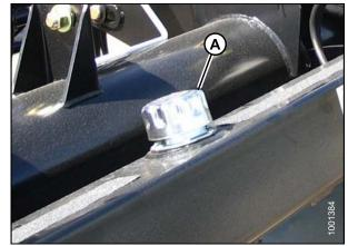
Figure 5.32: Oil Reservoir Filler Cap
