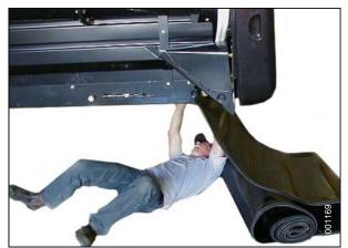
Figure 5.213: Installing Draper
