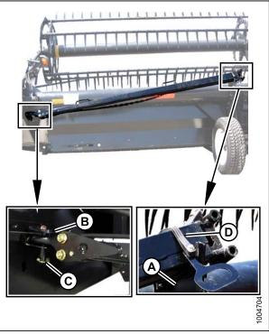
Figure 3.407: Tow-Bar Removal – Left Side
