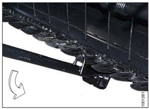
Figure 5.110: Downward Adjustment
