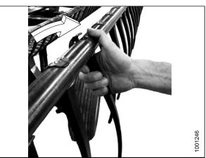
Figure 5.266: Installing Finger
