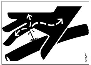
Figure 5.2: Hydraulic Pressure Hazard
