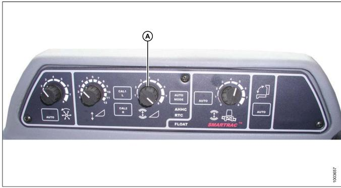
Figure 3.166: Auto Header Height Control Console
