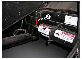
Figure 3.162: Combine Accumulator ON/OFF Switch A - Accumulator Lever (Off Position)
