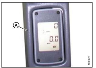
Figure 3.167: Tachometer
