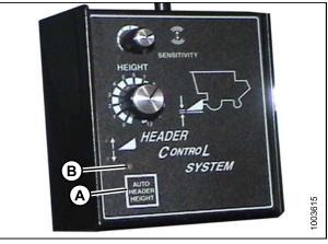
Figure 3.152: Combine Header Control System
