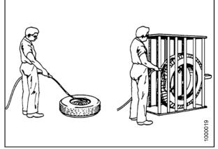
Figure 1.15: Safely Filling a Tire with Air
