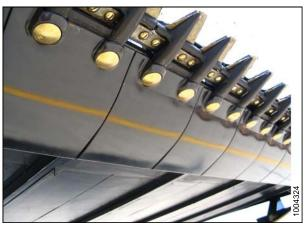
Figure 6.6: Cutterbar Wear Plates
