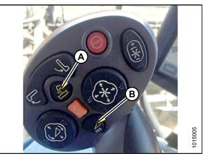
Figure 3.344: New Holland Combine Controls
