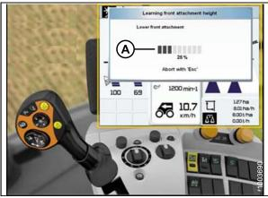
Figure 3.314: Lexion Combine Display, Console, and Joystick
