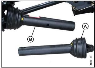
Figure 5.43: Separated Driveline
