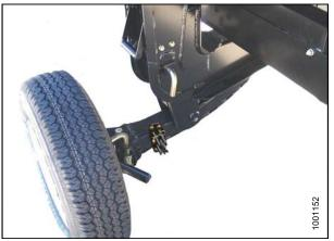
Figure 3.402: Left Wheel in Transport Position
