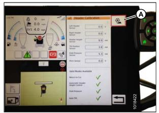
Figure 3.191: Header Calibration
