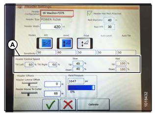
Figure 3.184: Header Speed Control Settings
