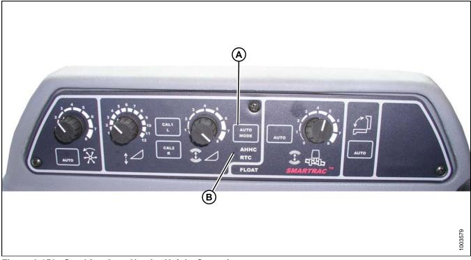
Figure 3.159: Combine Auto Header Height Controls
