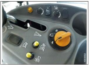
Figure 3.143: Height Adjustment Knob on the Combine Control Console
