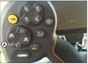
Figure 3.190: Header Down Switch
