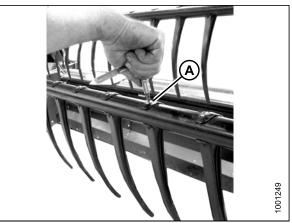
Figure 5.267: Installing Finger
