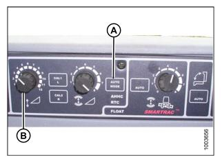
Figure 3.164: Auto Header Height Control Console
