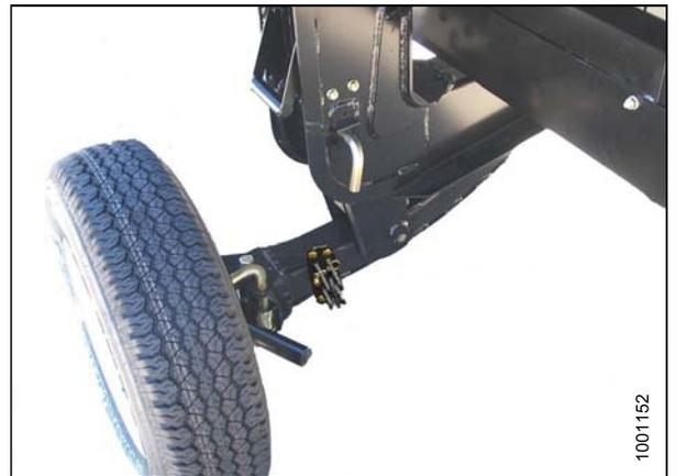
Figure 3.103: Left Wheel in Transport Position
