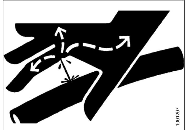
Figure 5.3: Hydraulic Pressure Hazard
