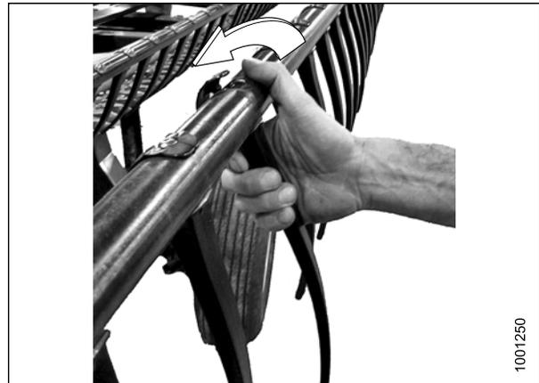
Figure 5.161: Removing Plastic Fingers
