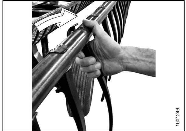
Figure 5.162: Installing Finger
