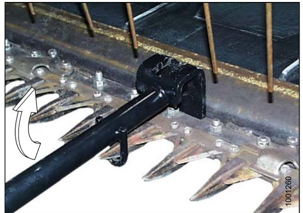
**Figure 5.33: Upward Adjustment**
