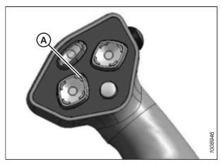
Figure 10.13: Ground Speed Lever (GSL)
