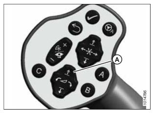
Figure 10.10: Ground Speed Lever
