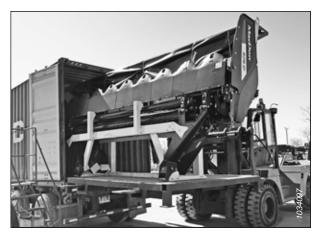
Figure 3.6: Rotary Disc Header in Container
