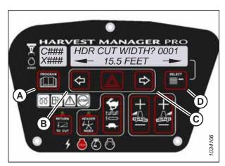
Figure 5.107: M205 SP Windrower Header Cut Width
