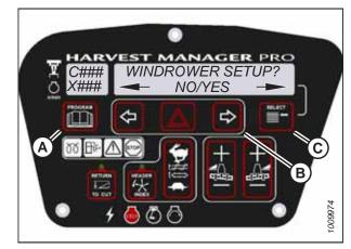
Figure 5.106: M205 SP Windrower CDM Programming Buttons
