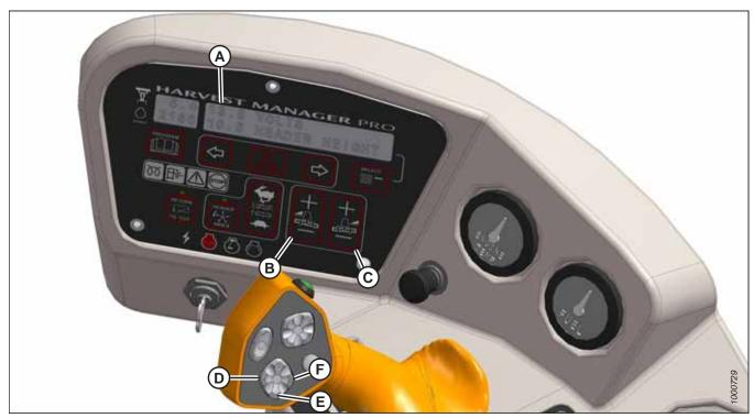
Figure 9.11: Cab Display Module (CDM) Float Adjustment
