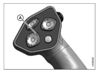
Figure 5.88: Ground Speed Lever
