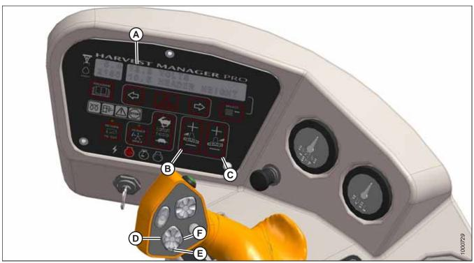
Figure 9.13: Cab Display Module (CDM) Float Adjustment
