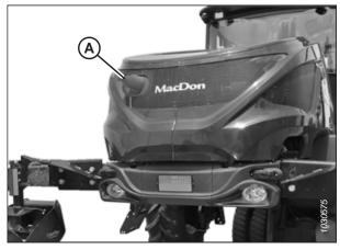
Figure 10.1: Engine Exhaust
