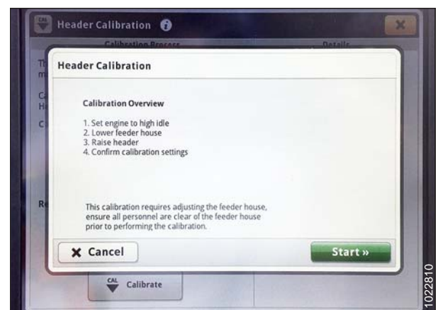
Figure 3.343: John Deere S7 Display – Header Calibration
