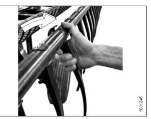
Figure 4.294: Installing Plastic Finger
