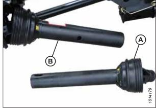
Figure 4.51: Separated Driveline
