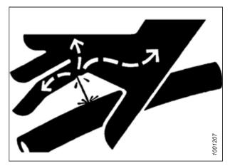
Figure 1.12: Hydraulic Pressure Hazard
