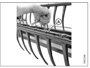
Figure 4.295: Installing Plastic Finger
