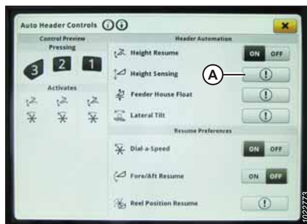
Figure 3.703: John Deere S7 Display – Auto Header Controls
