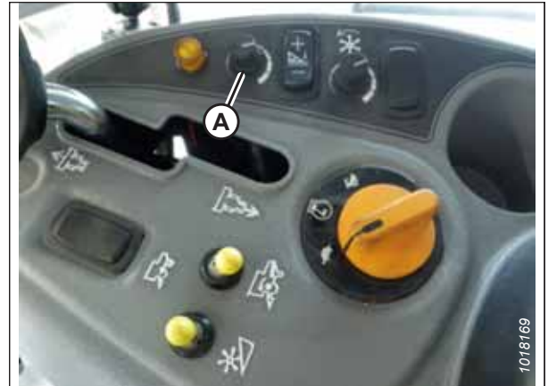
Figure 3.484: Height Adjustment Knob on the Combine Control Console
