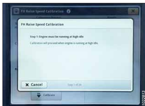
Figure 3.716: John Deere S7 Display – Feeder House Calibration
