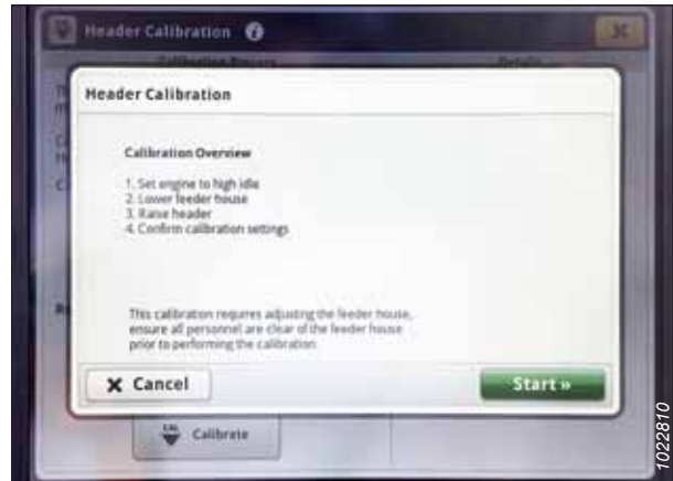
Figure 3.723: John Deere S7 Display – Header Calibration
