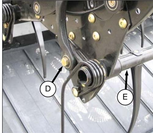
2. Remove bolt (D) at on cam linkage so that tine tube (E) is free to rotate.
