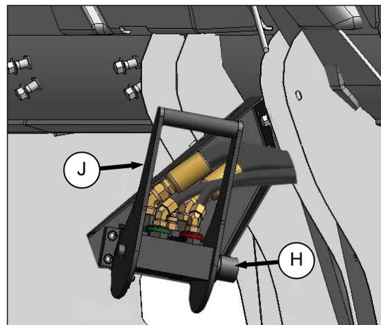
1. Push in lock button (H), and pull handle (J) up to "one-half open position".
