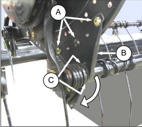
1. Remove bolts (A) securing arm (B) to disc.
