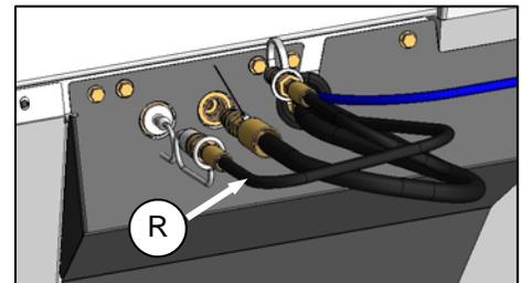
6. Disconnect reel fore-aft hoses (Q) and (R) (red discs) from combine and adapter receptacles.
