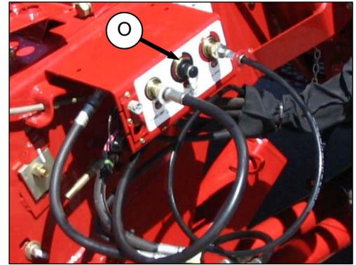
4. Remove plug from reel lift coupler (O) (black disc) on combine.
