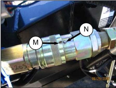
1. Line up slot (M) in collar with pin (N) on connector.
