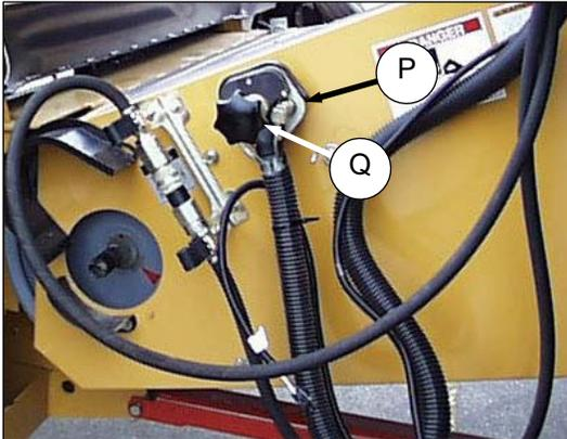
6. Locate coupler onto combine receptacle (P), and turn knob (Q) to secure coupler to receptacle.
