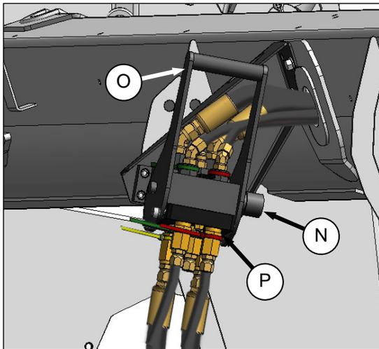
3. Position coupler (P) from combine onto receptacle, and push handle (O) to engage pins on coupler.
