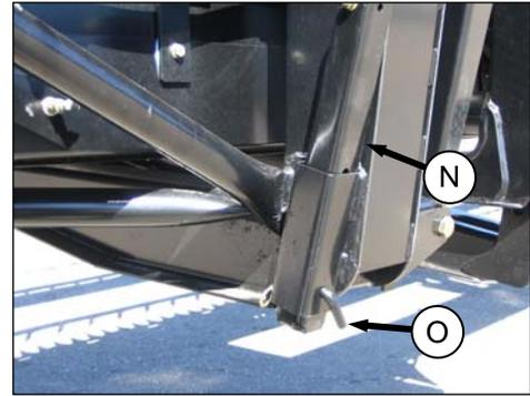
3. Return stand (N) to “storage position”, and secure with pin (O).
