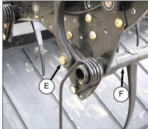
1. Remove bolt (E) at on cam linkage so that tine tube (F) is free to rotate.
