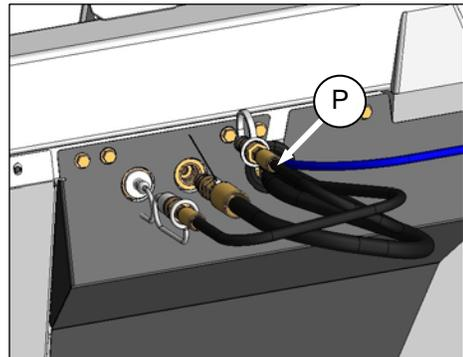
4. Disconnect reel lift hose (P) (black disc) on combine, and attach red dust cap. Store hose on adapter.
