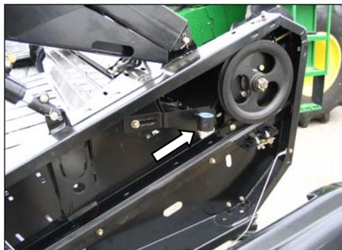
A spare sickle may be stored in the header frame tube at the left end (as shown above). Ensure sickle is secured in place.
