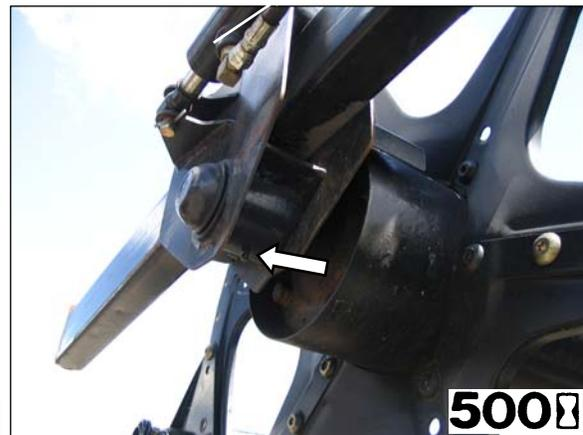
REEL SHAFT LH BEARING (1 PLC)
