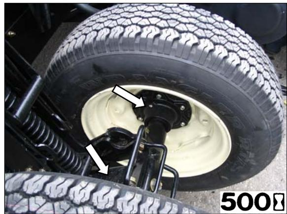
WHEEL BEARINGS (2 PLC BOTH SIDES)
