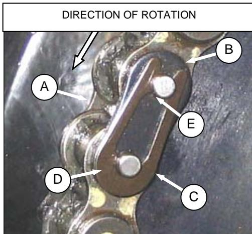
3. Install pin connector (A) (not available as a MacDon part) into chain, preferably from sprocket backside.
