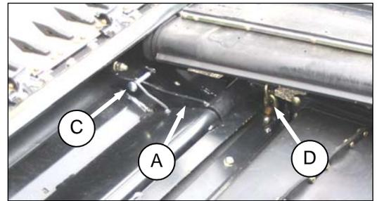
1. Rotate latch (A) with a 15/16 wrench (or equivalent) on hex (B) to raise feed deck so that bolt (C) can be removed. Repeat for other side of feed deck.
