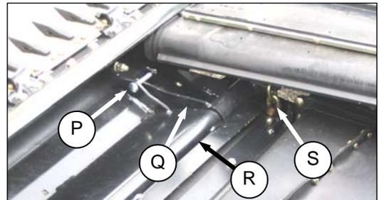
1. If installed, remove bolts (P) at either side of opening to allow attachment of adapter deck.
