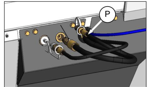
5. Remove red dust cap from reel lift hose (P) on adapter, and connect hose to combine coupler (O).
