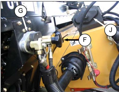
3. Clean mating surface of coupler (G), and locate onto adapter receptacle. Turn knob (F) to secure coupler to receptacle.
