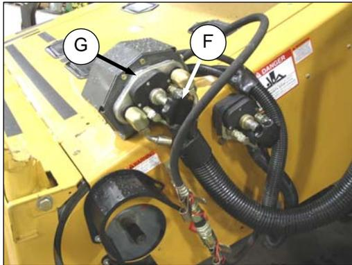
3. Locate coupler (G) onto combine receptacle, and turn knob (F) to secure coupler to receptacle.
