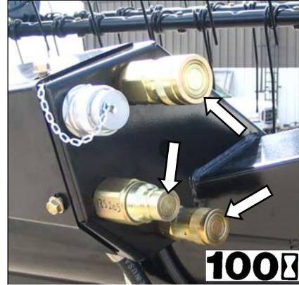
LUBRICATE WITH WD40® OR EQUIVALENT
