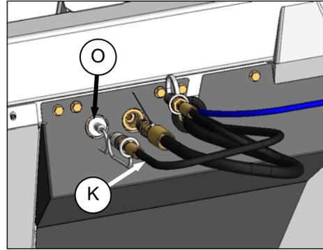
3. Connect hose (K) from the adapter to the adapter coupler (O).
