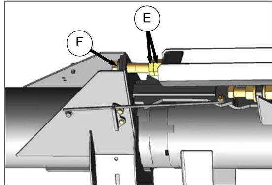
**Condition 1:** Unlock nuts (E), and turn bolt (F) until edges are parallel. Lock nuts (E).
