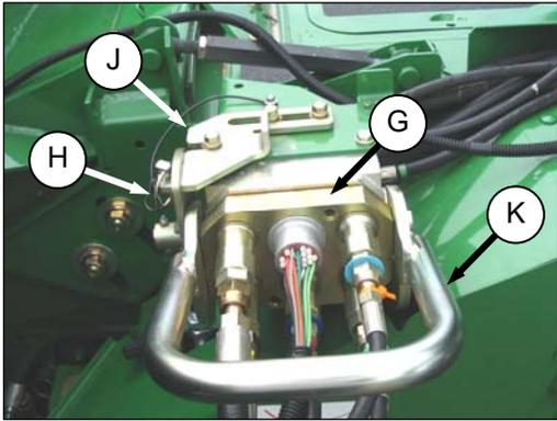
1. Remove lynch pin (H), and slide lock (J) to release handle (K).
