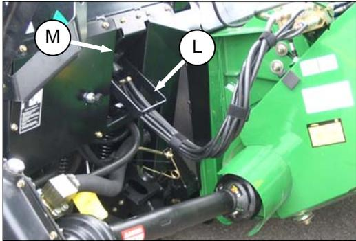
3. Lift handle (L) on adapter, position coupler in adapter at (M), and lower handle (L) to lock coupler.
