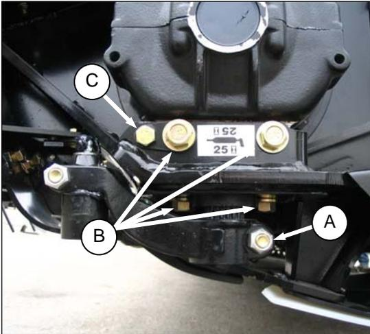
Check four wobble box mounting bolts (B) torque after the first 10 hours operation, and every 100 hours thereafter. Torque should be 200 ft-lbf (270 N·m).
