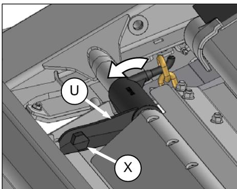
3. Rotate latch (U) with a 15/16 wrench (or equivalent) on hex (X) to raise feed deck so that bolt (T) can be re-installed. Repeat for other side of feed draper.
