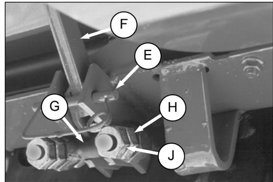
3. Remove pin (E), and lower latch handle (F) (one on each side of feeder house underside) to hook latch (G).
