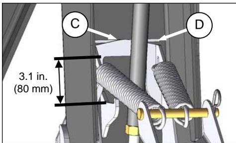
**Condition 2:** The top of the balance link (C) is lined up with the white decal strip (D) within 1/2 in. (12 mm).
