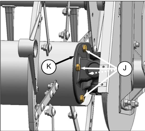
2. Remove four bolts (J) attaching reel tube to U-joint (K).
