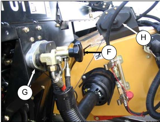
1. Unscrew knob (F) on coupler (G) to release coupler from adapter.
