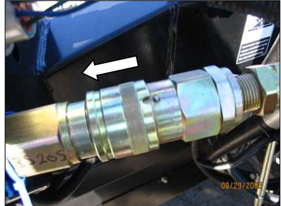
3. Push hose connector onto mating receptacle until collar on receptacle snaps into lock position.
