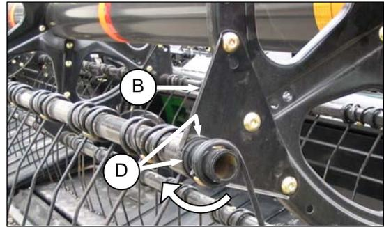
3. Rotate arm (B) clear of disc, and slide arm inboard off bushing, and remove bushing halves (D). Remove bolt from tine next to arm (or remove plastic finger) if required so that arm can slide off bushing.
