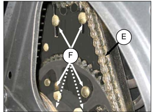
2. Route new chain (E) over U-Joint (K), and locate on sprockets.
