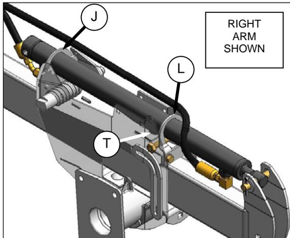
3. Lift the aft end of the cylinder out of support assembly, and move the cylinder so that cylinder center port fitting (T) engages the support assembly.
