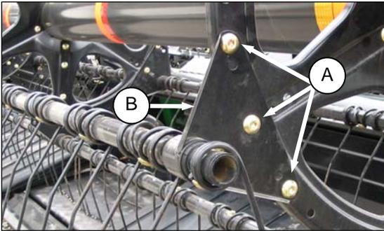
1. Remove bolts (A) securing arm (B) to disc at both locations.
