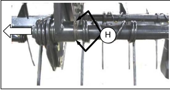
3. Slide tine tube to expose bushing. Remove bushing halves (H).
