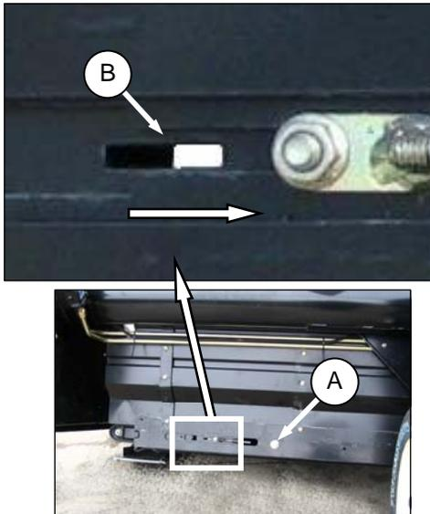
indicator bar (B) will move inboard in direction of arrow (indicating that draper is tightening). Tighten until bar is about "halfway" in window.
