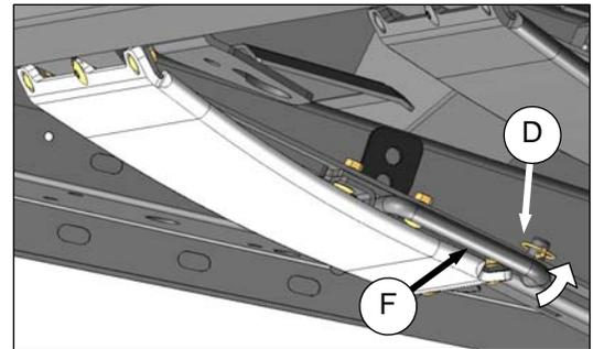
4. Re-insert pin (F), engage in frame, and secure with lynch pin (D).
