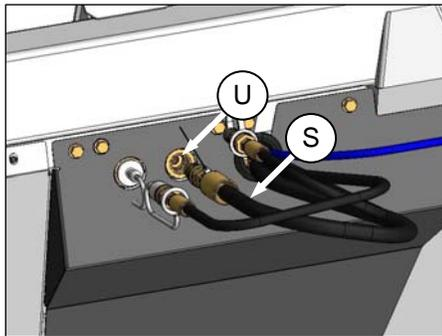
8. Connect hose (S) from the adapter to the adapter coupler (U).
