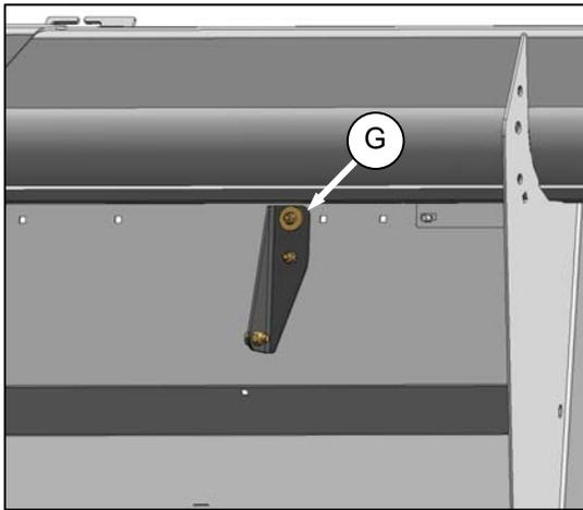
1. Remove support (G) from backsheet, and remove hardware from support. Retain hardware.
