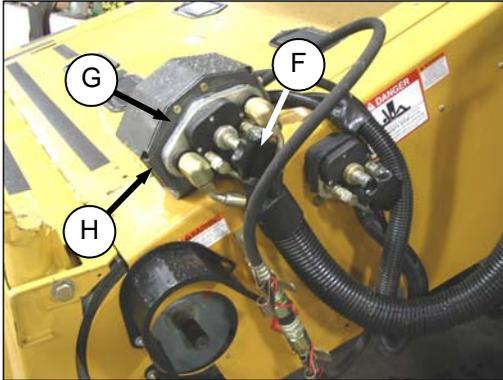
1. Unscrew knob (F) on combine coupler (G) to release coupler from combine receptacle (H).
