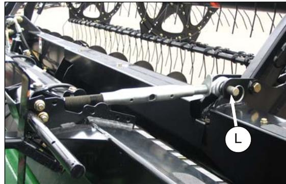
1. Remove pin (L) to release link. Replace pin.
