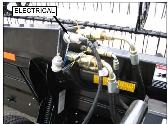
2. Align lugs on connector with slots in receptacle, push connector onto receptacle, and turn collar on connector to lock it in place.
