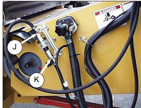
2. Disconnect hydraulic hoses from adapter connectors (L) and (M). Locate hoses (J) and (K) on combine as shown, and re-connect.
