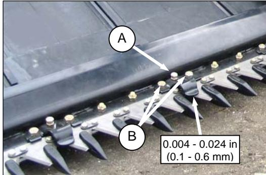
1. Turn the adjuster bolts (A). Using a feeler gauge, clearance from hold-down to sickle section should be 0.004 - 0.024 in. (0.1 - 0.6 mm).
