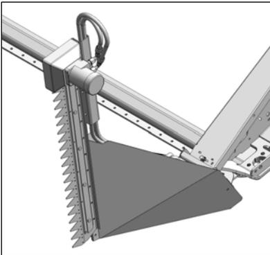
The vertical knife mounts allow installation of vertically oriented sickles onto both ends of D50, D60, and FD70 headers.
