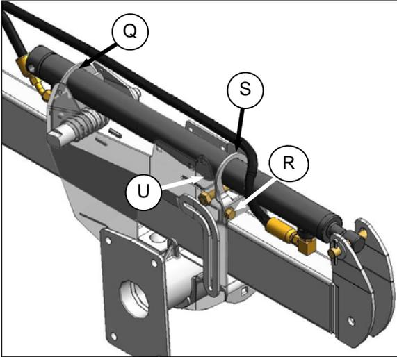
5. Lift aft end of the cylinder out of the support assembly, and move cylinder so that cylinder center port fitting (U) engages the support assembly.
