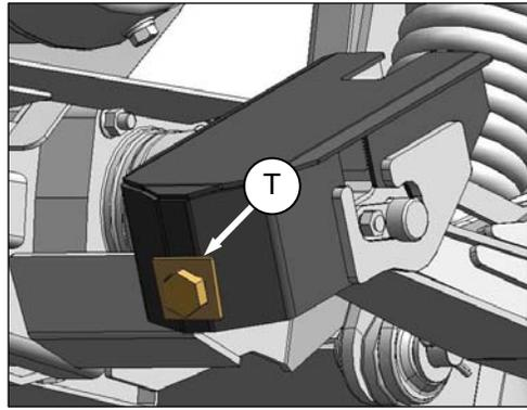
w. Re-install bolts (T), washers, and spacers removed in step k. into adapter legs.
