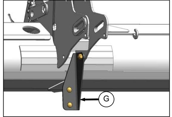
3. After deck is moved, attach backsheet to support (G) with hardware provided.
