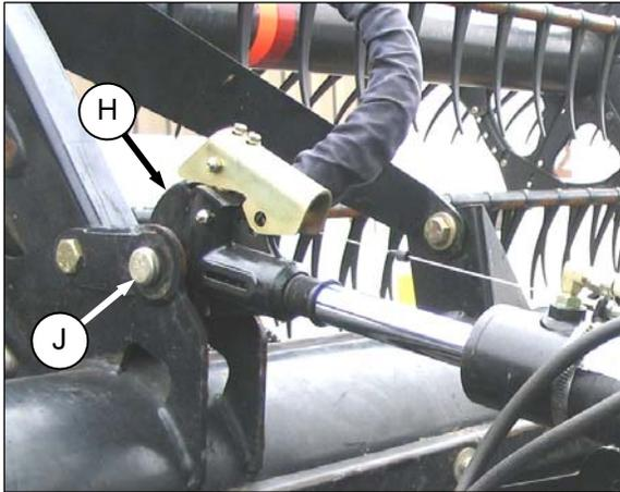
1. Extend hook (H), and remove prop under link so that base of hook rests on pin (J).
