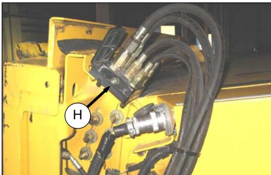
3. Remove hydraulic quick coupler (H) from storage plate on combine, and clean mating surface of coupler.
