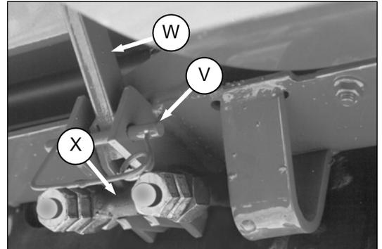
2. Remove pin (V), and lower latch handle (W) (one on each side of feeder house) to disengage latch (X).
