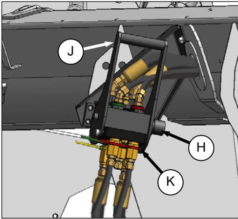
3. Position coupler (K) from adapter onto receptacle, and push handle (J) to engage pins on coupler.
