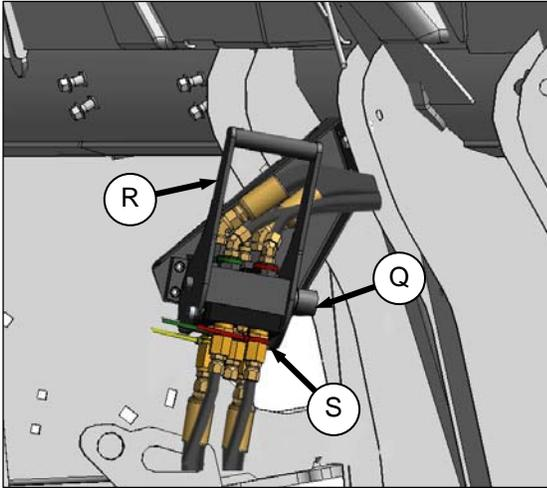
1. Push in lock button (Q), and pull handle (R) to release coupler (S).
