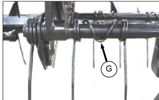
2. If required, remove bolt (G) securing the first tine to the left of the support so that tine is free to move inboard (to the right). If plastic finger is installed, refer to previous section for removal procedure.
