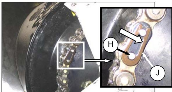
3. Rotate auger to expose connector link (H).
