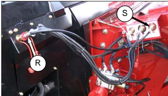
6. Disconnect reel fore-aft hoses (R) and (S) (red discs) from adapter and combine receptacles.
