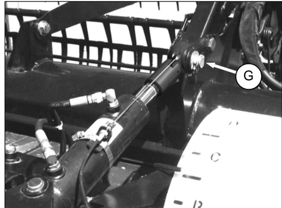
4. Insert pin (G), and secure with lynch pin.
