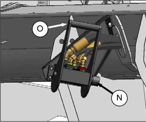
1. Push in lock button (N), and pull handle (O) to "full open position".
