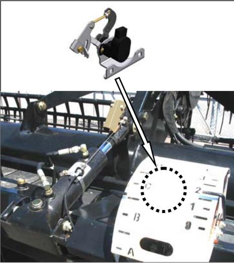
For use in conjunction with Auto Header Height Control option on Case, New Holland, John Deere and AGCO combines, and with the Header Float option on Lexion combines on Model D50 and D60 Harvest Headers. It is standard equipment on the FD70 FlexDraper header.
