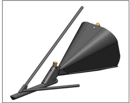
Optional special rice dividers can be installed and used when required. See Section 12.15 RICE DIVIDER KIT.
