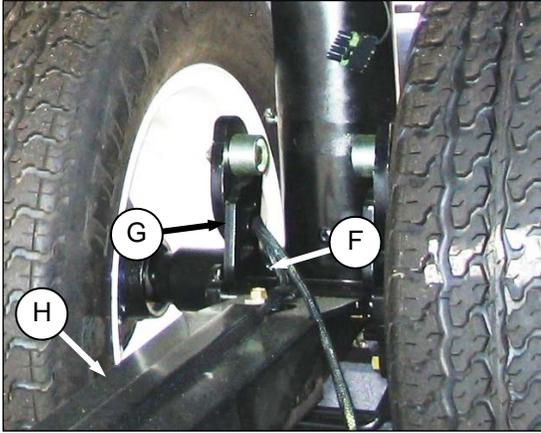
4. Remove clevis pin (F), and set aside for later installation.
