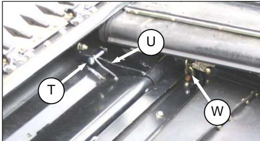
1. If installed, remove bolts (T) at either side of opening to allow attachment of adapter deck.
