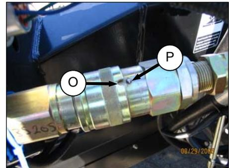
1. Line up slot (O) in collar with pin (P) on connector.
