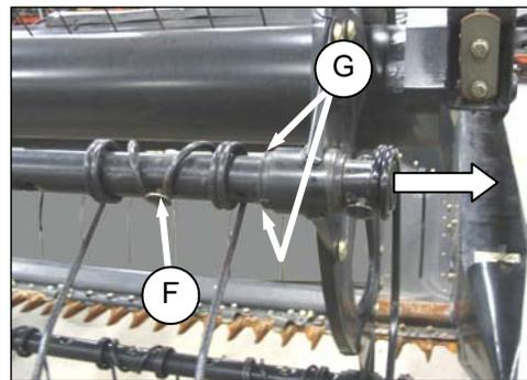
4. Remove bolt (F) from tine (or remove plastic finger) next to arm if required so that tube can slide through arm.
