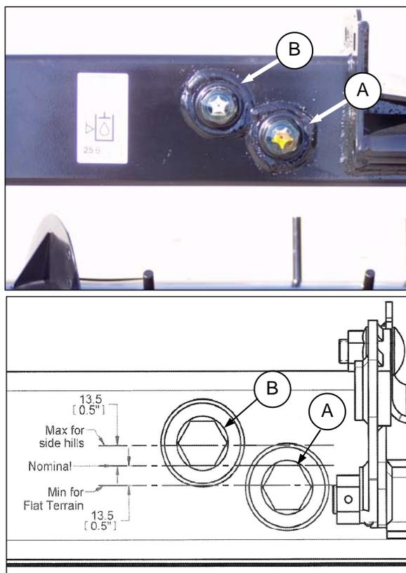
Check oil level every 25 hours at sights (A) and (B) with cutterbar just touching ground. Check when oil is cold, and with center-link retracted.
