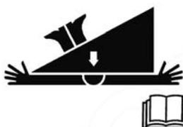
**Rest header on ground or engage mechanical locks before going under unit. See Operators Manual.**
