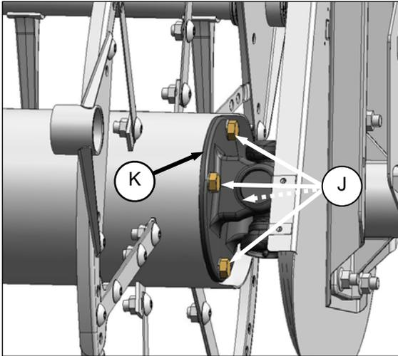
5. Position RH reel tube against reel drive, and engage stub shaft into U-joint (K) pilot hole.
