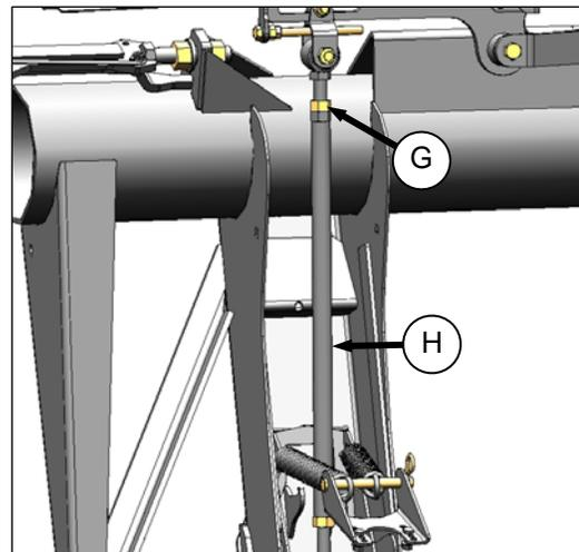
**Condition 2:** Unlock jam-nut (G) and turn compression link (H) until balance link (C) and decal (D) are lined up, or the dimension is met. Lock the nut (G).
