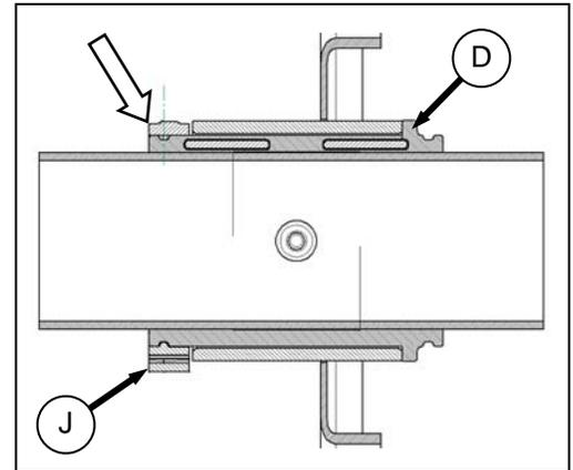
1. Spread clamp (J), and slip over tine tube adjacent to flangeless end of bushing.
