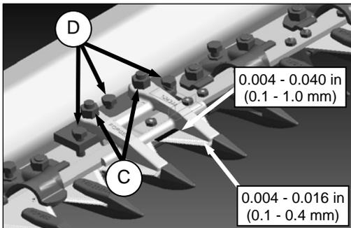
1. Torque nuts (C) to 35 ft·lbf (46 N·m).
