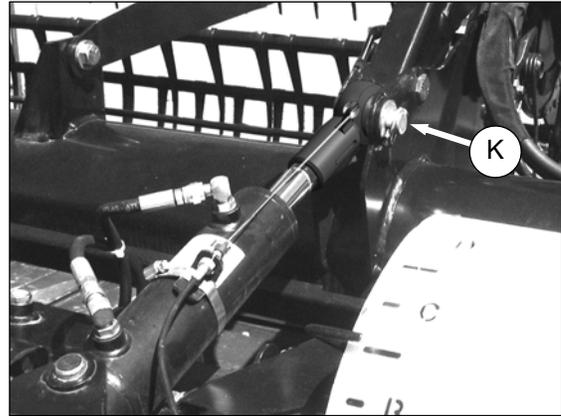
1. Operate center-link hydraulics until pin (K) is loose.
