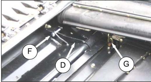
3. Rotate latch (D) with a 15/16 wrench on hex (E) to raise feed deck so that bolt (F) can be removed. Repeat for other side of feed draper deck.
