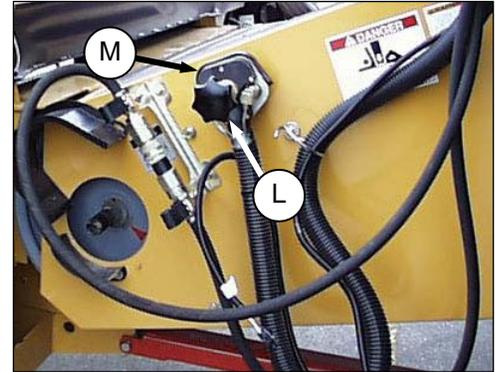
1. Unscrew knob (L) on combine coupler (M) to release coupler from combine receptacle.
