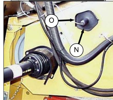
2. Remove cover (N) from adapter receptacle, and place on combine receptacle (O).
