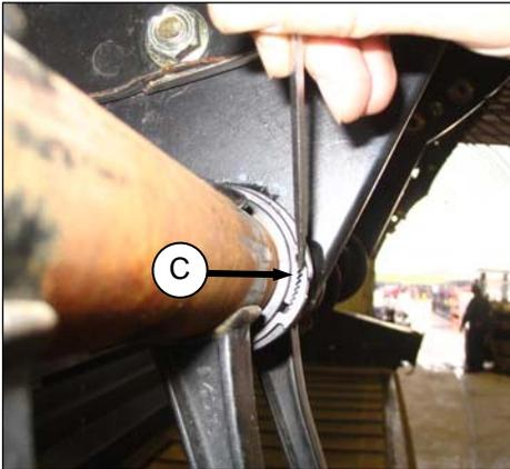
2. Release bushing clamps (C) using a small screwdriver to separate the serrations. Pull clamp off tine tube.
