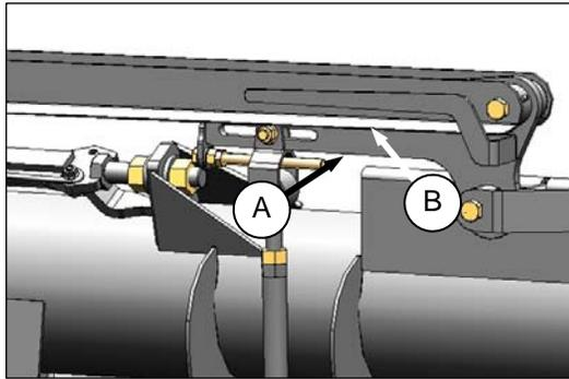
**Condition 1:** Bottom edge of bellcrank (A) is parallel to the bottom edge of the center-link (B).
