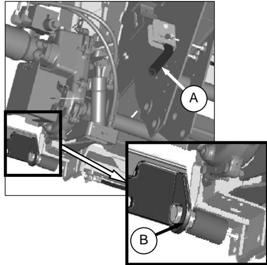
4. Lower handle (A) to engage pins (B) into adapter.
