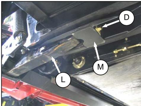
2. Install bolts (D), spacers and lock washers removed at step c. to secure adapter arms (L) to header legs (M).
