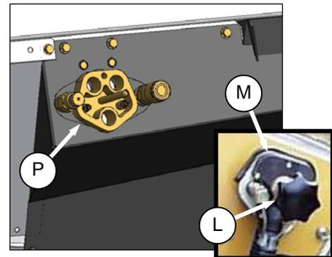
3. Locate combine coupler (M) onto adapter receptacle (P), and turn knob (L) to secure coupler to receptacle.
