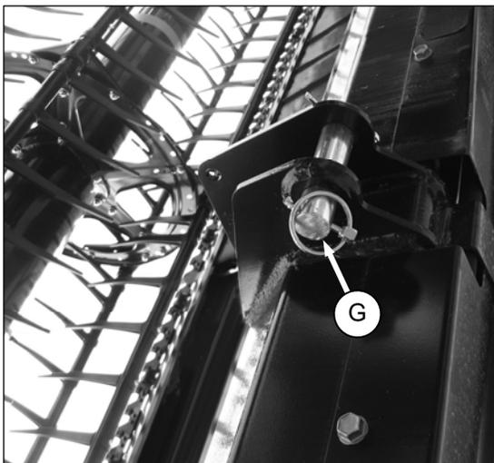
2. Remove pin (G), and the prop under link.
