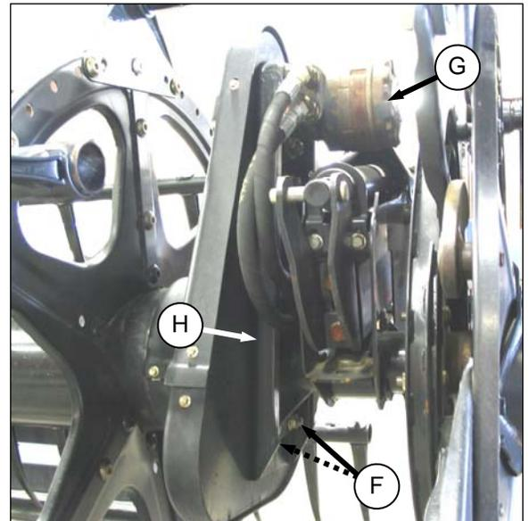
3. Slide motor (G) and motor mount (H) until tension on chain is such that hand force deflects chain 1/8 inch (3 mm) at mid-span.
