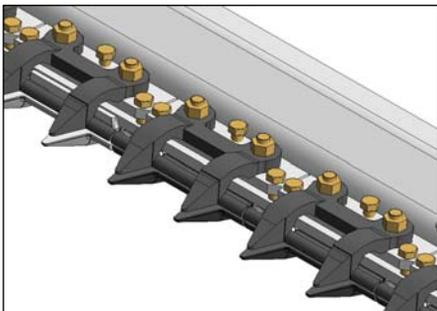
Stub guards, complete with top guides and adjuster shoes are designed to cut tough crops.
