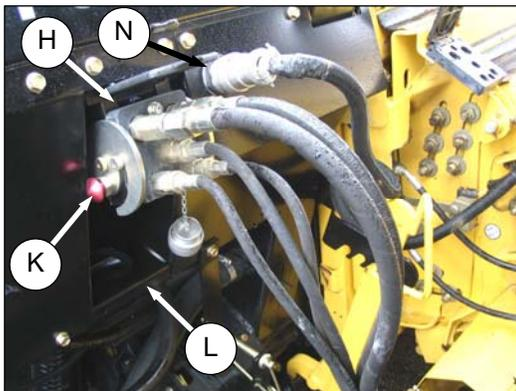
4. Position coupler onto adapter receptacle (M), and push handle (L) to engage pins into receptacle.
