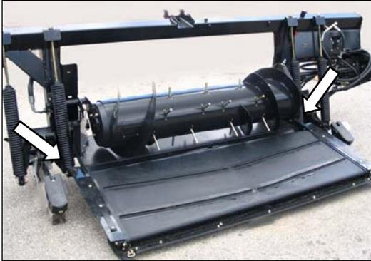
There is a drain plug at the bottom of each side frame.
