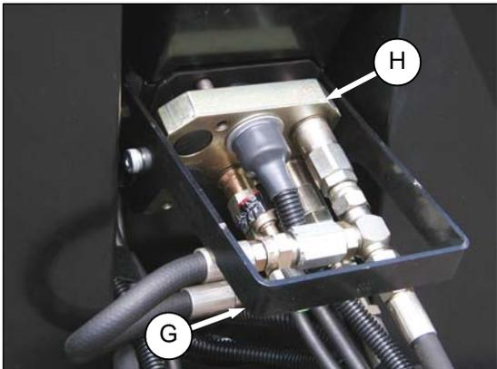
2. Lift handle (G) on adapter, position coupler (H) in adapter, and lower handle (G) to lock coupler.
