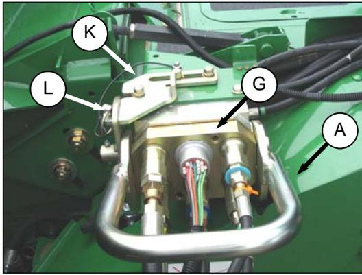
2. Locate coupler (G) onto receptacle, and pull handle (A) so that lugs on coupler are engaged into handle.
