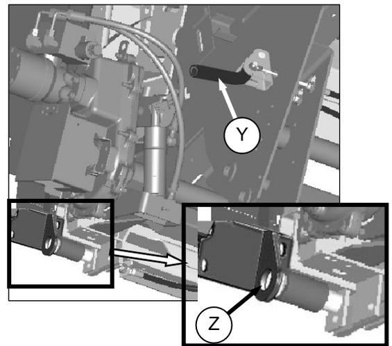
1. Raise handle (Y) on left side of feeder house to retract pins (Z).
