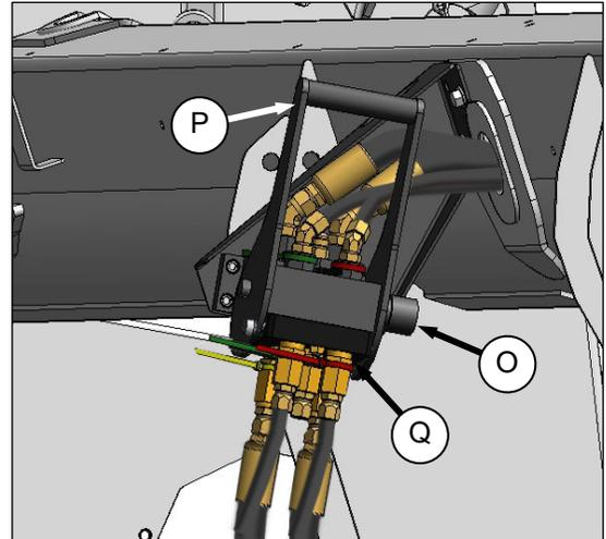
1. Push in lock button (O), and pull handle (P) to release coupler (Q).
