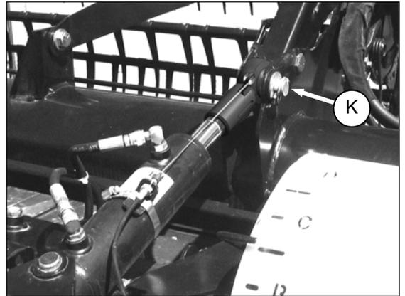
4. Insert pin (K), and secure with lynch pin.
