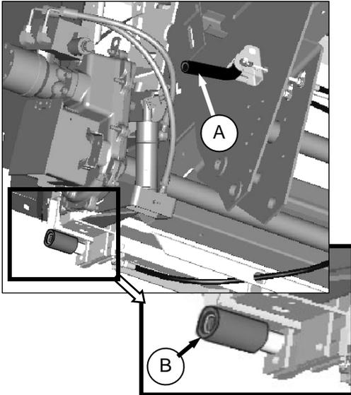
1. Move handle (A) on left side of feeder house to up position to retract both pins (B) at lower corners of feeder house.
