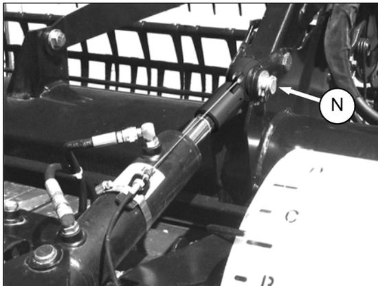
1. Remove pin (N), and lift center-link clear of bracket.
