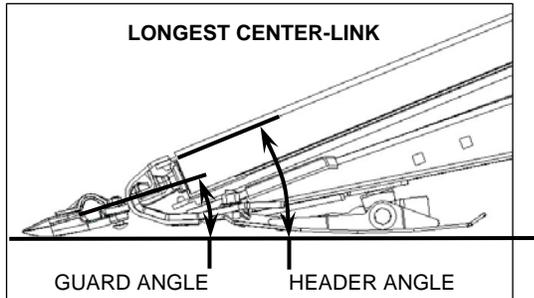
Flatter header angles are recommended for normal crop conditions and for stony ground because it minimizes sickle section breakage and reduces soil scooping or build-up at the cutterbar in wet conditions.
