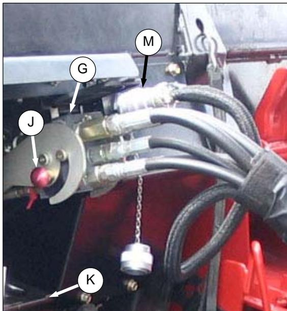
4. Position onto adapter receptacle (G), and push handle (K) to engage coupler pins into receptacle.
