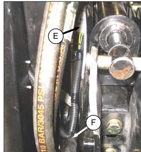
2. Disconnect connector (E), and cut plastic tie (F) securing harness to hose.
