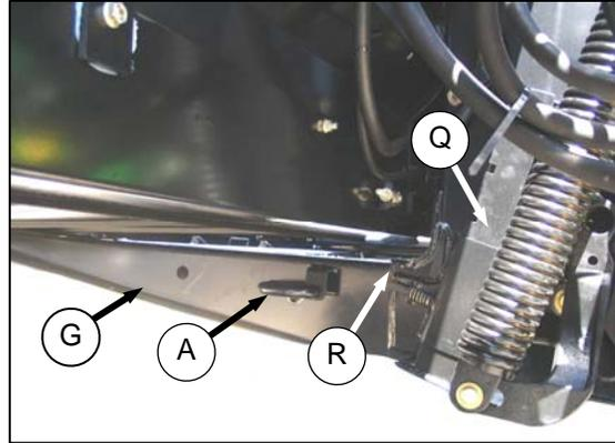
1. Ensure adapter arm is properly located in header leg (G). Re-install pin (A) in each leg to lock header to adapter, and secure with lynch pin.
