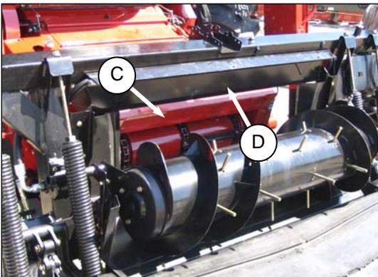
2. Slowly drive combine up to adapter until feeder house saddle (C) is directly under the adapter top cross member (D).
