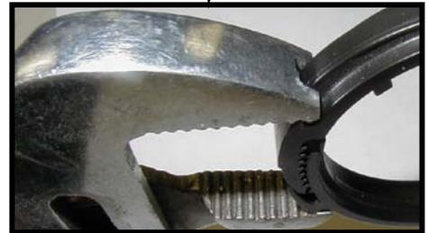
3. Tighten clamp with modified channel lock pliers (K) so that finger pressure will not move clamp.
