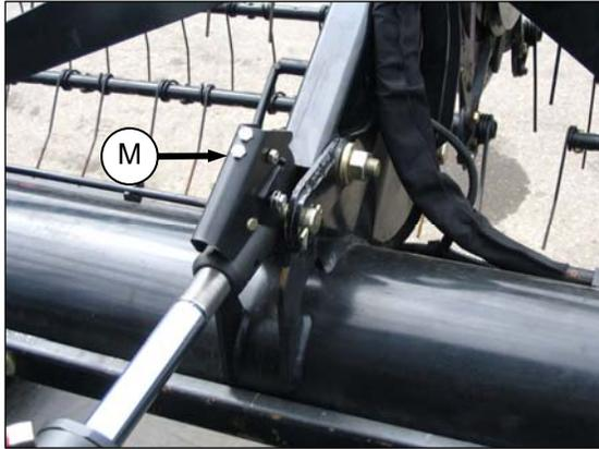
1. Lift release (M), and latch it in "up position".
