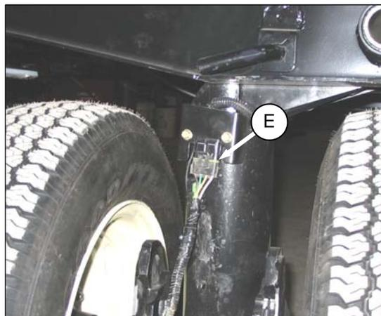
3. Disconnect wiring connector (E) at front wheel.
