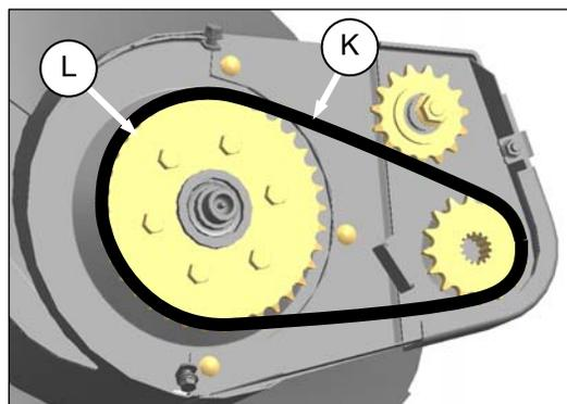
CUTAWAY VIEW OF CHAIN CASE
