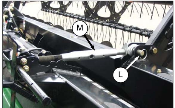
2. Remove pin (L) and the prop under link.
