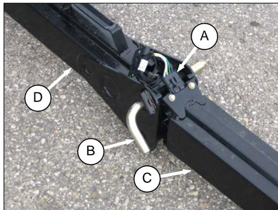
1. Disconnect wiring connector (A) on tow-bar.
