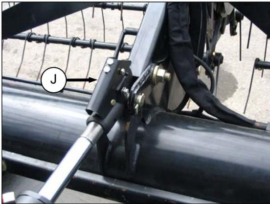
1. Lift release (J) and latch it in "up position".
