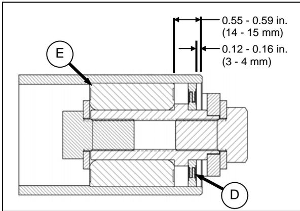
1. Install bearing assembly (E) into roller by pushing on outer race of bearing. The bearing is fully positioned when the 0.55 inch (14 mm) dimension is achieved.
