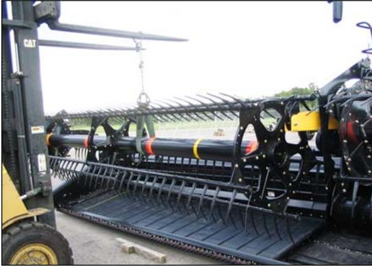
1. Support inboard end of right reel with a front end loader and nylon slings (or equivalent set-up).
