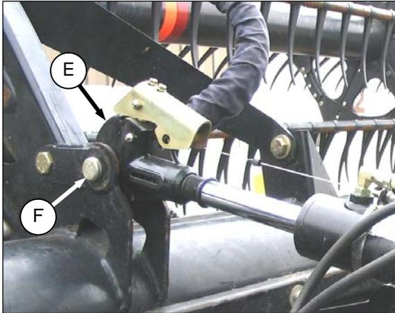
1. Extend hook (E), and remove prop under link so that base of hook rests on pin (F).
