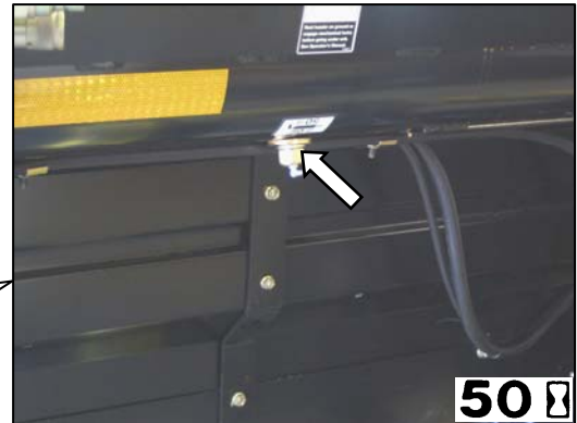
KNIFE DRIVE SHAFT - DK (BOTH SIDES) 15 PUMPS MINIMUM
