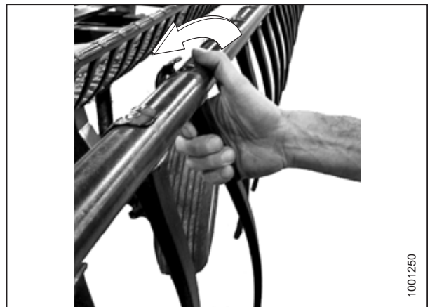
Figure 5.177: Removing Plastic Finger
