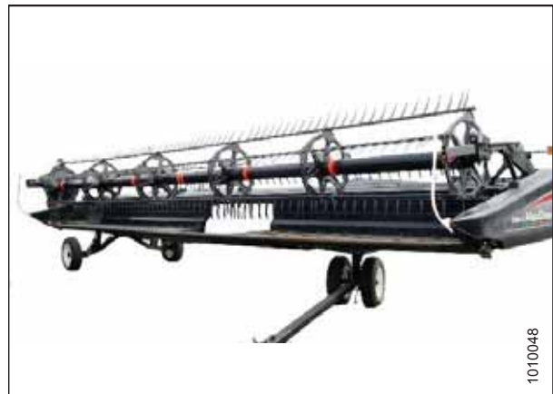
Figure 6.15: Stabilizer Wheels and Transport
