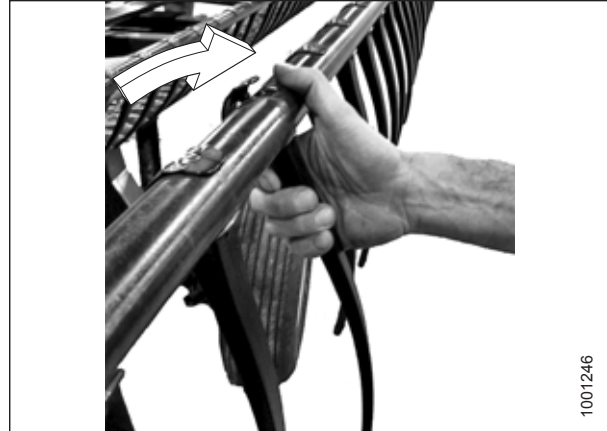
Figure 5.178: Installing Plastic Finger
