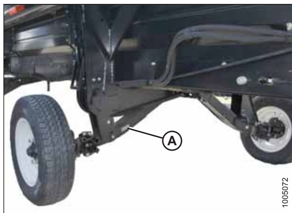
Figure 3: Transport / Stabilizer Wheel Location
