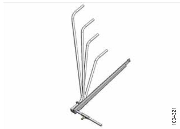
Figure 6.22: Swath Forming Rods
