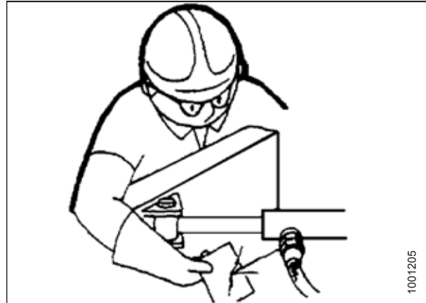
Figure 1.11: Testing for Hydraulic Leaks
