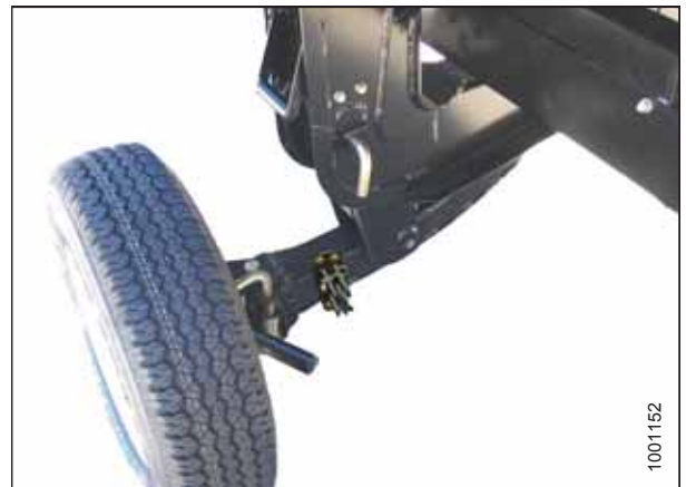
Figure 3.79: Left Wheel in Transport Position
