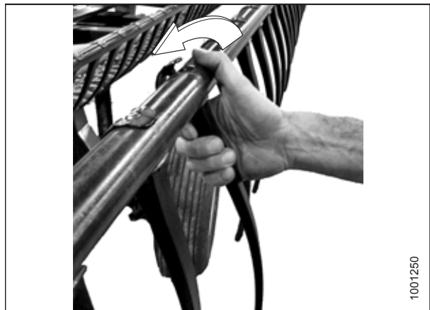
Figure 5.166: Removing Plastic Fingers
