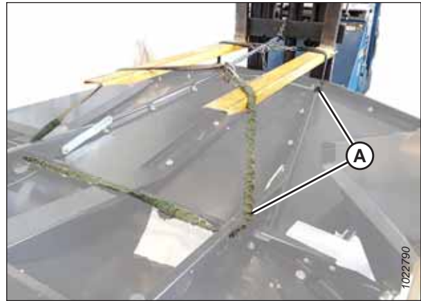
Figure 2.31: Lifting Swath Compressor Shield
