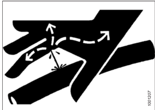
Figure 1.12: Hydraulic Pressure Hazard
