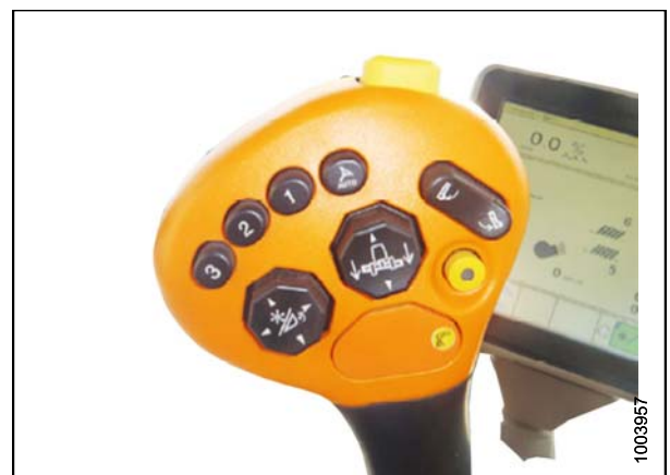
Figure 8.112: Use the Joystick to Set the Ground Pressure Presets
