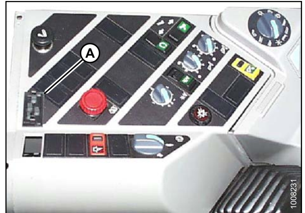
Figure 6.83: Switch Plug in Console
