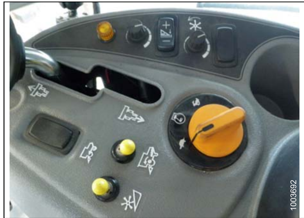
Figure 8.18: Height Adjustment Knob on the Combine Control Console
