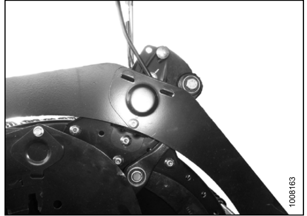
Figure 6.132: Right-Hand Reel with Cam Arms Attached
