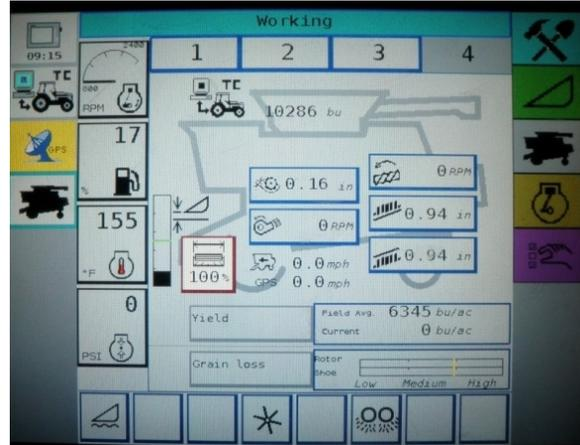
To select the AHHC mode, scroll through the header control options using the header control switch until the AHHC icon is displayed in the first message box.
