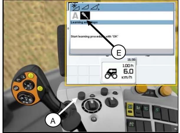
7. Raise the feeder house all the way up. This will allow the graph to go to 33% (F).
