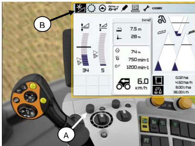
3. If you are not using Auto Reel Speed, in the window under *Reel*, select *Reel speed* (C). A graph displays. Use control knob (A) to adjust the reel speed.
