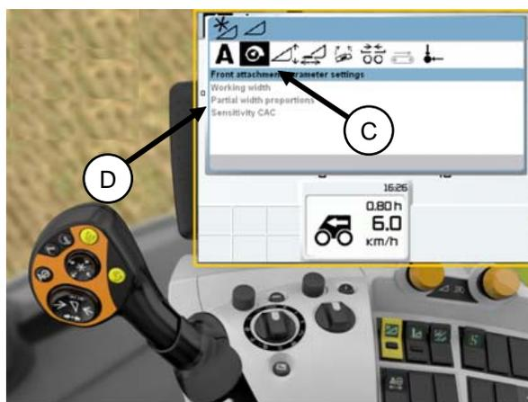
5. To set the sensitivity you will have to change the cutting height adjustment from the 0 default. The settings between 1 to 50 provide a faster response. Settings between -1 to -50 provide a slower response. When making adjustments to the above numbers, do it in increments of 5.
