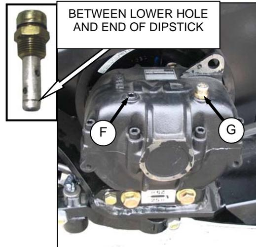
KNIFE DRIVE BOX (CHECK OIL LEVEL WITH TOP OF KNIFE DRIVE BOX HORIZONTAL)
