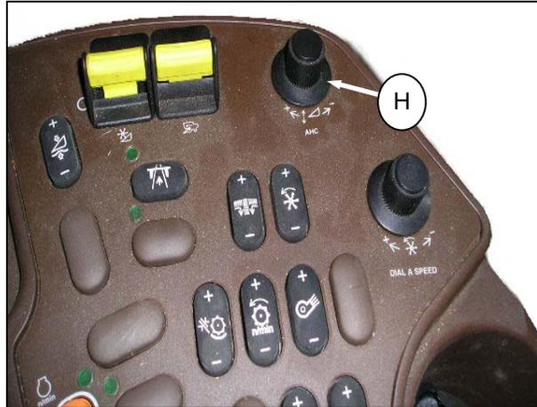
**NOTE:** Desired ground pressure is in most cases one number separation of the Auto Header Height from having the header fully suspended off the ground (D) to just sitting on the ground (C).
