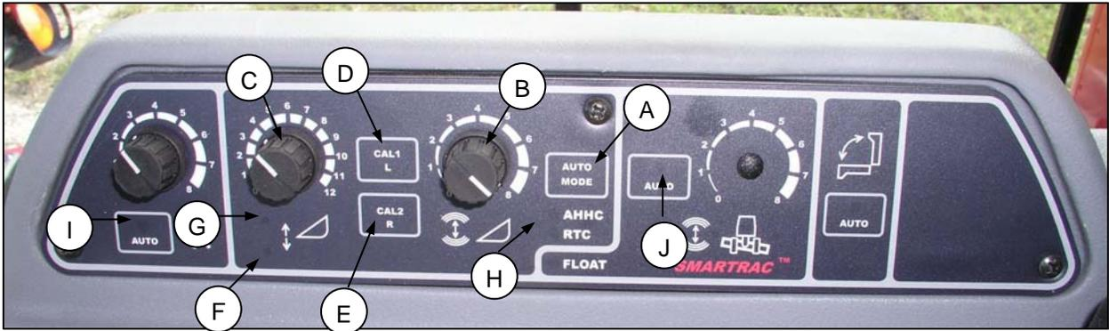
2. Press and hold CAL1 button (D) until you see the following lights flash: header (G) (F), tilt auto mode (J) and AHHC (H).
