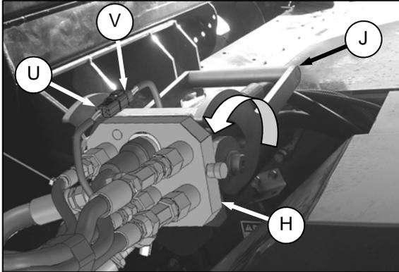
4. Position coupler (H) onto combine receptacle (K), and pull handle (J) to fully engage coupler into receptacle.
