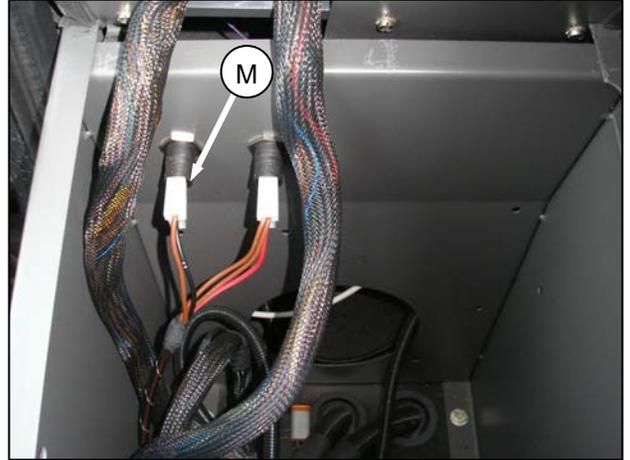
2. Replace the plug with the black wire (N) on the top terminal, and red wire (P) to bottom terminal.
