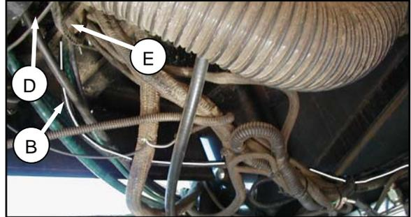
ROUTE HARNESS INTO CAB AT ELECTRICAL PLATE
