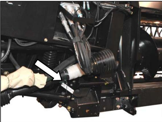
l. Remove shipping wire from driveline and float lock lever.
