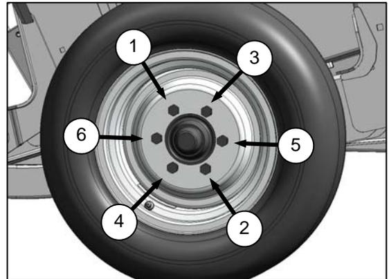
Check wheel bolt torque is 80–90 lb-ft (110–120 N·m). Refer to bolt tightening sequence illustration above.
