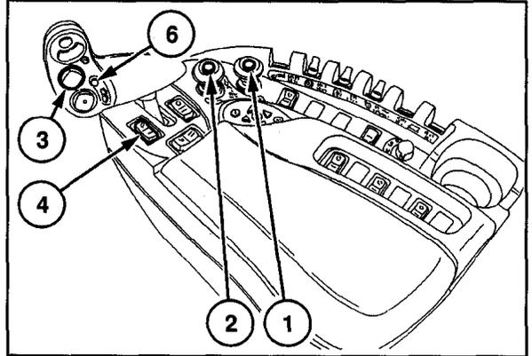
6. To change one of the memorized header height setpoints during working, using the header height and header lateral floatation rocker switch, 3, (slow up/down) to raise or lower header to the desired value. Press the automatic header height control button, 6, for a minimum of 2 seconds to store the new height position. (A beep will confirm setting).
