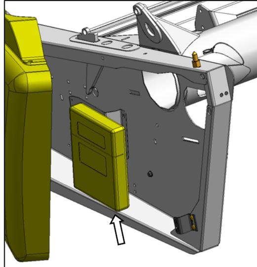
Check case contents. The manual case is located inside the LH endshield.
