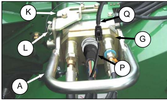
2. Locate coupler (G) onto receptacle, and pull handle (A) so that lugs on coupler are engaged into handle.
