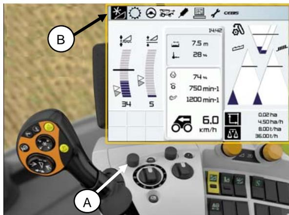
2. The following screen will show up with **A** highlighted. Scroll right using the control knob (A) to highlight the icon of the header with up & down arrows behind it (C).
