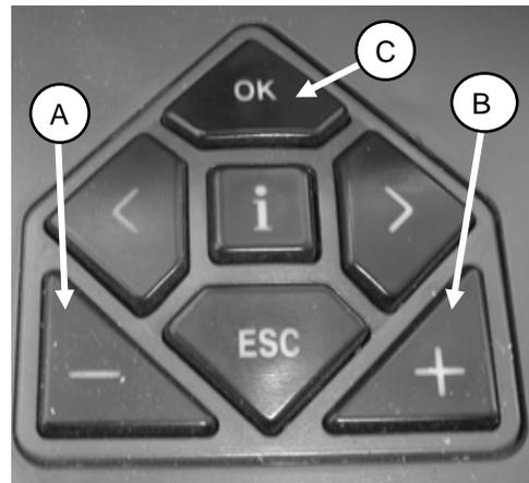
You can also manually adjust the reel speed by rotating the rotary switch to the reel position (D), and then using the “-” key (A) or the “+” key (B) to set the reel speed.
