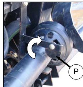
j. Rotate disc (P) on adapter driveline storage hook, and remove driveline from hook.
