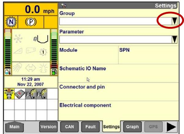
4. Select *Header Height/Tilt*. The Parameter window opens.
