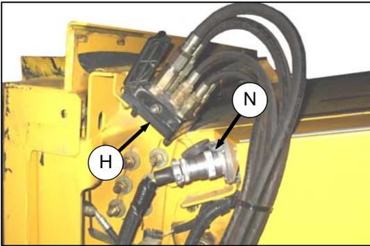
3. Remove hydraulic quick coupler (H) from storage plate on combine.
