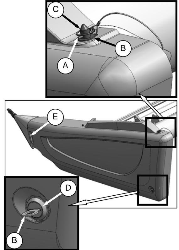
2. Remove lynch pin (A), and tool (B) from pin (C) at top rear of endshield.
