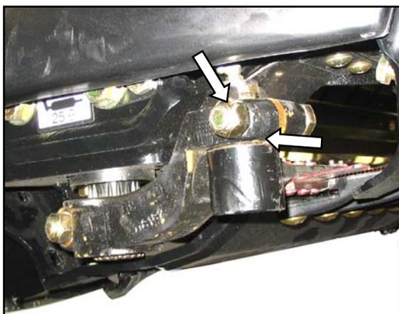
1. Check gap between knifehead and pitman arm. A business card should slide easily through the gap. If not, then adjust gap by loosening bolt and tapping knifehead with a hammer. Retighten bolt.
