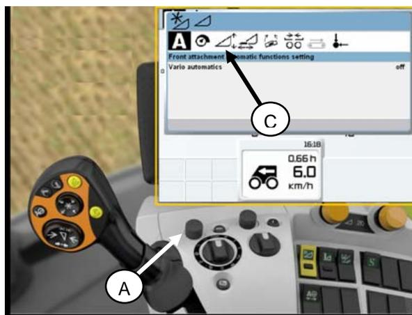
3. When the header with up and down arrows is highlighted push control knob (A). The following screen will show up with the header icon highlighted (D).
