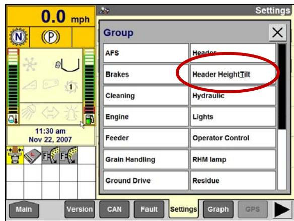
5. Select *Left header height sen*, and then select the *Graph* button at the bottom of the screen. The exact voltage is displayed at top of screen.
