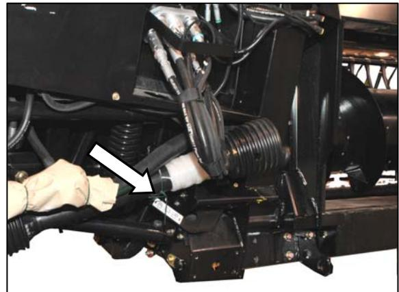
k. Remove shipping wire from driveline and float lock lever.
