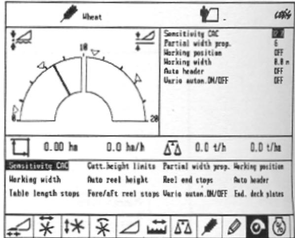
Line (A) indicates the setting of the sensitivity. Window E4 (B) displays the (A). Also value (C) indicates the sensitivity. Window E5 (D) displays value (C).
