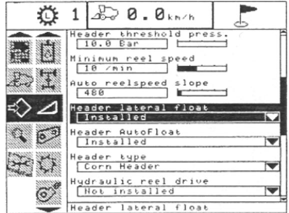
3. On the combine display screen, select *Header Autofloat*, and then press ENTER.
