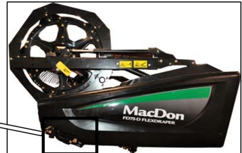
To prevent binding and/or excessive wear caused by knife pressing on guards, do **NOT** over grease. If more than 6 to 8 pumps of the grease gun are required to fill the cavity, replace the seal in the knifehead.
