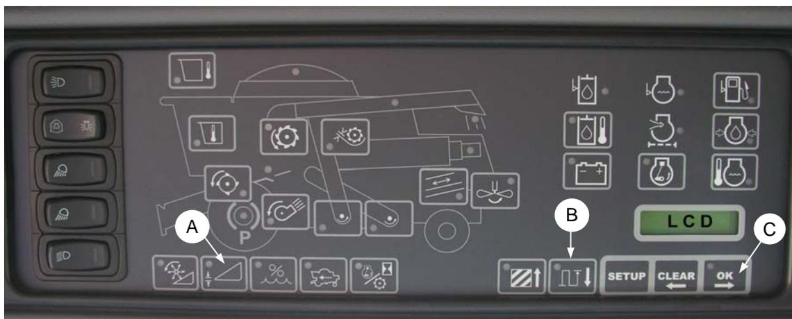
2. Scroll down using button (B) until "LEFT" is displayed on the LCD screen.
