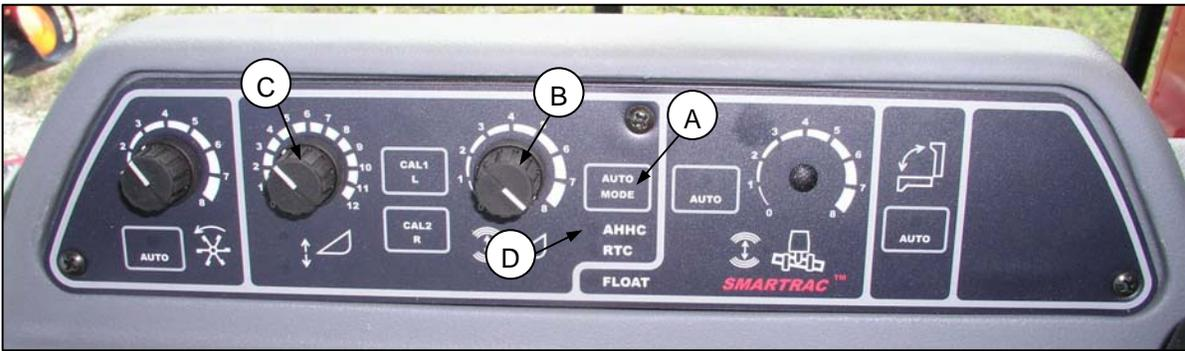
2. Momentarily press the down button (E) on the control handle. The AHHC light (D) should change from flashing to solid. The header should also drop toward the ground. The Auto Header Height control is now working and active and can be adjusted for height and sensitivity.
