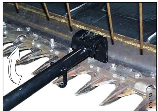
Figure 7.2: Straightening Tool – Upward Adjustment
