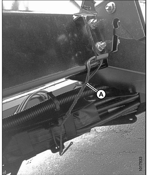
**Figure 3.6: Hose Management Arm in Shipping Position (12.2–13.7 Meter [40–45 Foot] Headers)**
