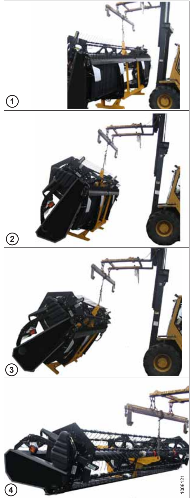
Figure 2.10: Lowering the Header
