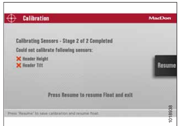
Figure 6.64: Sample of Failed Calibration Display Message
