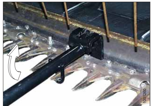
Figure 8.2: Straightening Tool – Upward Adjustment
