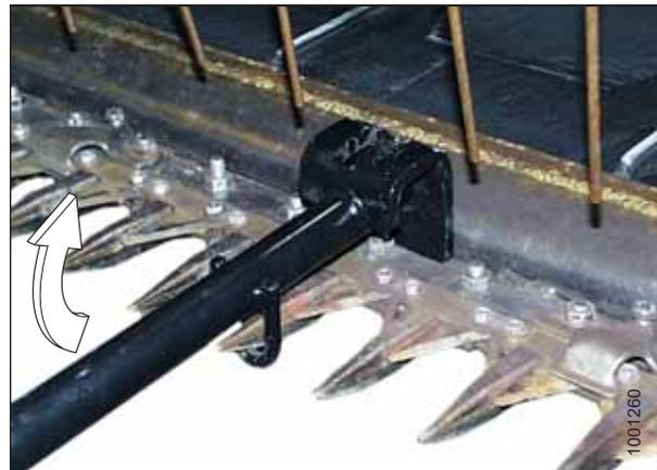
Figure 6.2: Straightening Tool – Upward Adjustment
