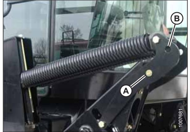
Figure 4.10: Float Springs Engaged
