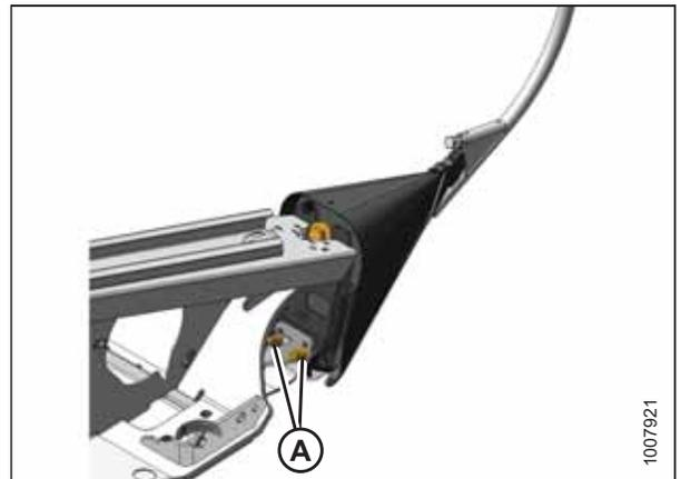
Figure 3.36: Adjustment Hardware
