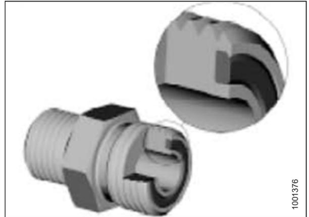
Figure 7.9: Hydraulic Fitting
