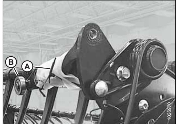
Figure 3.23: Cam Arm in Shipping Position
