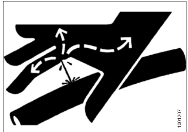
Figure 5.3: Hydraulic Pressure Hazard
