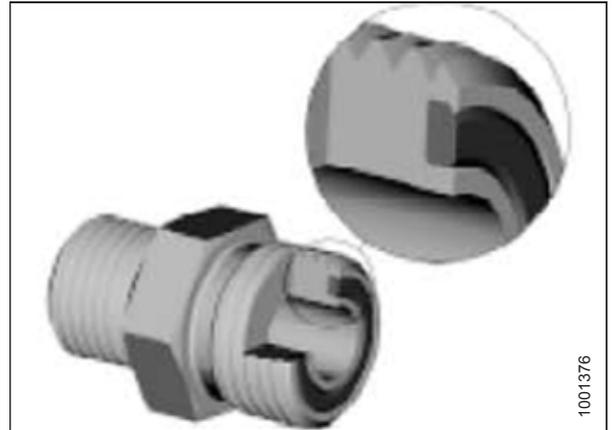
Figure 7.14: Hydraulic Fitting
