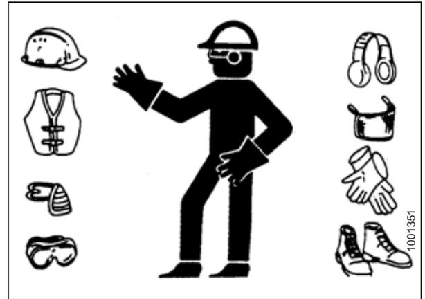
Figure 4.30: Protective Clothing and Personal Safety Devices
