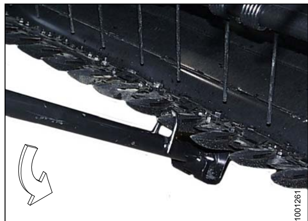
Figure 9.8: Guard Tips – Downward Adjustment
