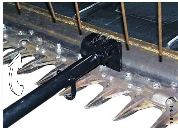
Figure 9.7: Guard Tips – Upward Adjustment
