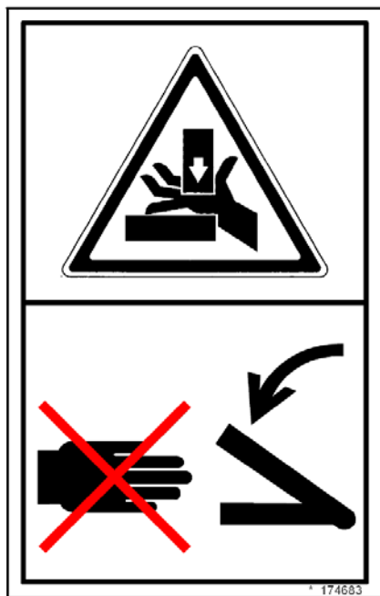
PART NO. 174683 PINCH POINT- MOVING PARTS STAND CLEAR LOCATED ON LINKAGE ARM (BOTH SIDES)
