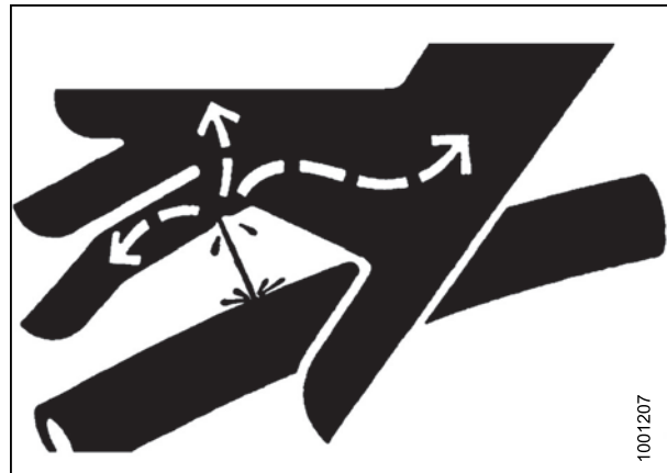
Figure 1.12: Hydraulic Pressure Hazard
