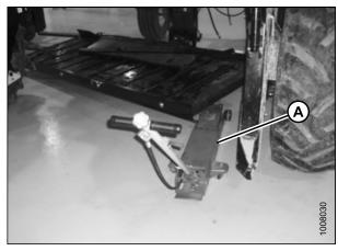
Figure 2.13: DWA Deck Supported with Floor Jack
