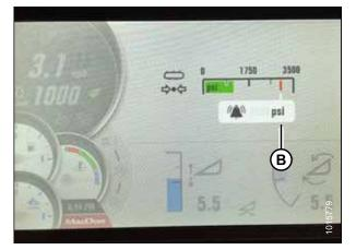
Figure 2.39: QuickMenu/Draper Pressure Alarm
