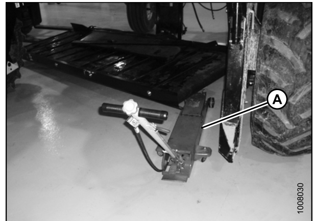
Figure 2.13: DWA Deck Supported with Floor Jack
