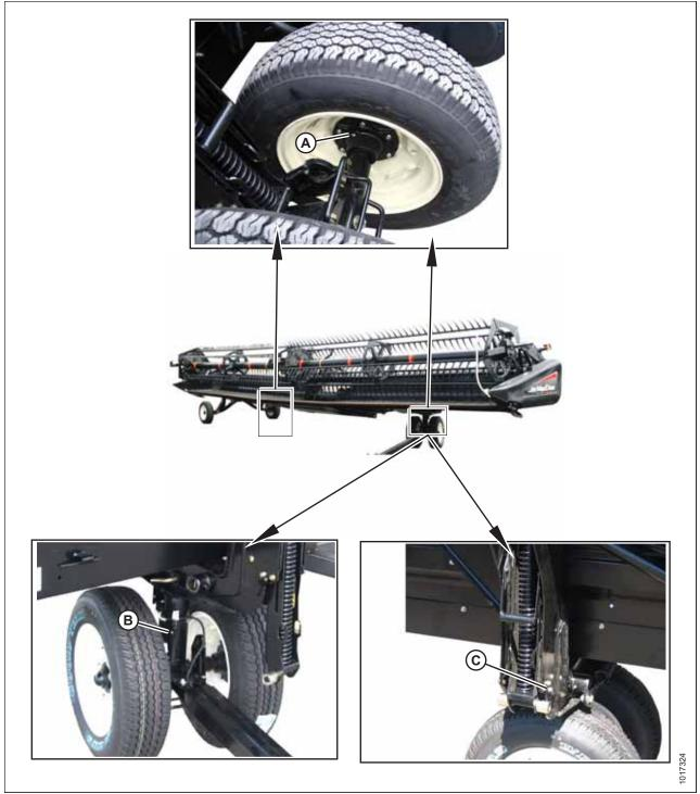
Figure 6.73: Rear Wheel Axle, Wheel Bearings, Frame/Wheel Pivot, and Front Wheel Pivot
