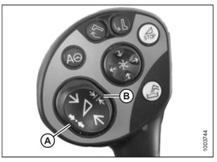
Figure 7.159: CLAAS Control Handle Buttons
