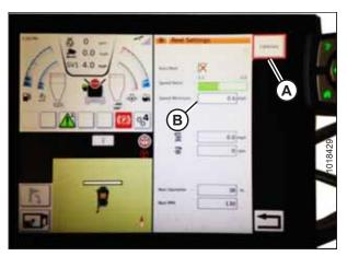
Figure 7.272: Reel Settings Calibration
