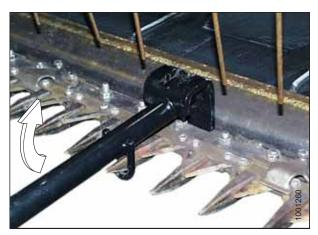
Figure 9.7: Straightening Tool – Upward Adjustment
