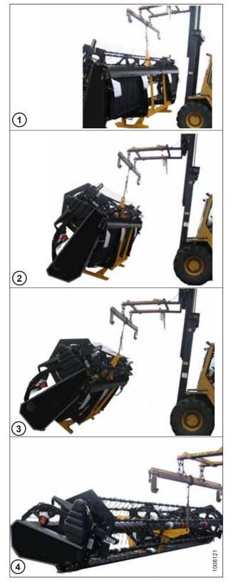
Figure 2.5: Header Lowered onto Ground
