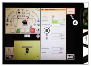
Figure 7.238: Reel Settings Calibration
