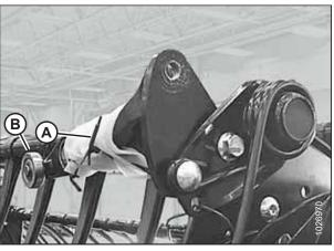
Figure 3.24: Cam Arm in Shipping Position
