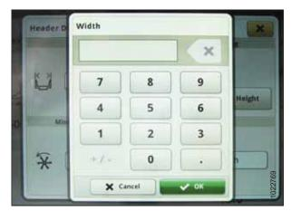
Figure 7.368: John Deere S7 Display – Setting Header Width
