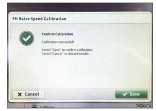
Figure 7.387: John Deere S7 Display – Feeder House Calibration
