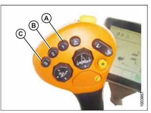
Figure 7.343: Control Handle Buttons
