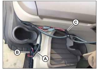
Figure 4.57: Harness Connections
