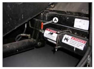
Figure 7.220: Combine Accumulator ON/OFF Switch A - Accumulator Lever (Off Position)
