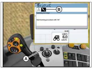
Figure 7.181: CLAAS Combine Display, Console, and Control Handle
