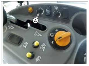
Figure 7.138: Height Adjustment Knob on the Combine Control Console
