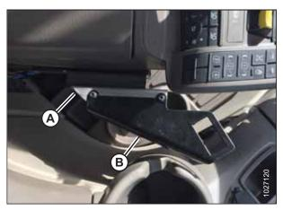
Figure 4.68: Top View of Armrest Showing Supports Installed in Alternative Location A - Tilt/Draper Speed Support B - Rocker Switch Support
