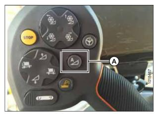
Figure 7.256: AHHC on Control Handle
