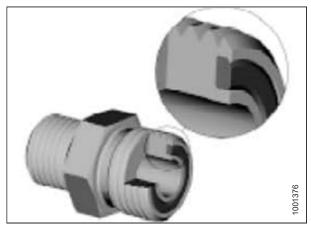
Figure 10.10: Hydraulic Fitting
