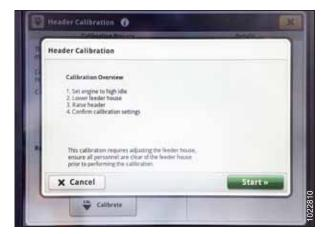
Figure 7.393: John Deere S7 Display – Header Calibration
