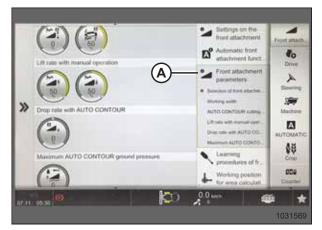
Figure 7.205: Front Attachment Parameters Page
