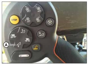
Figure 7.248: Header Down Switch
