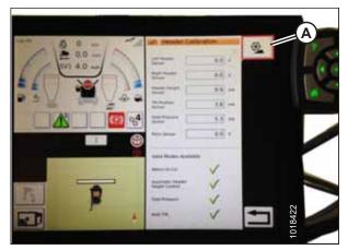
Figure 7.249: Header Calibration
