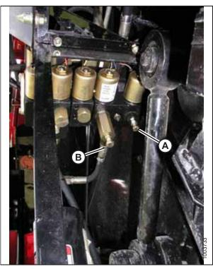
Figure 7.221: Header Raise and Lower Adjustable Restrictor's
