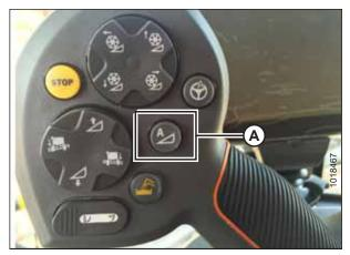
Figure 7.286: AHHC on Control Handle
