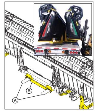
Figure 2.1: Header Shipping Supports
