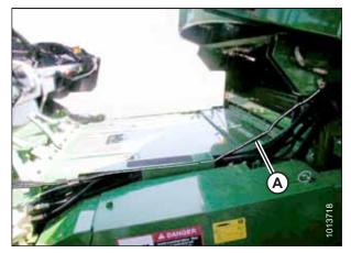
Figure 4.77: 60/70 Series Harness Routing
