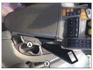
Figure 4.66: Top View of Armrest Showing Supports Installed in Preferred Location A - Tilt/Draper Speed Support B - Rocker Switch Support
