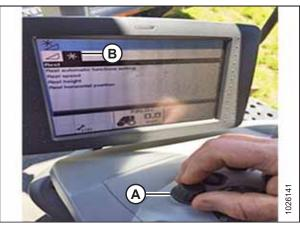
Figure 7.179: CLAAS Combine Display and Console
