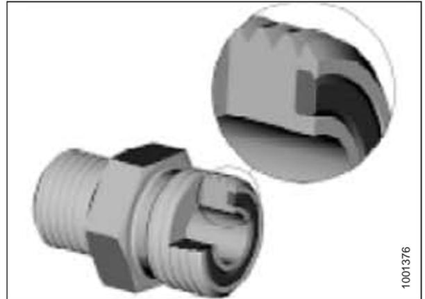
Figure 6.13: Hydraulic Fitting
