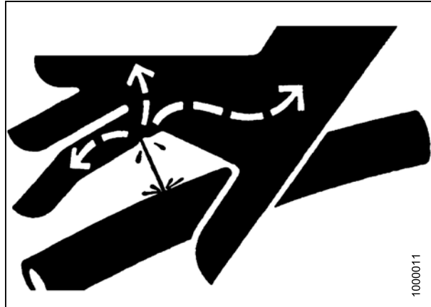
Figure 7.84: Hydraulic Pressure Hazard
