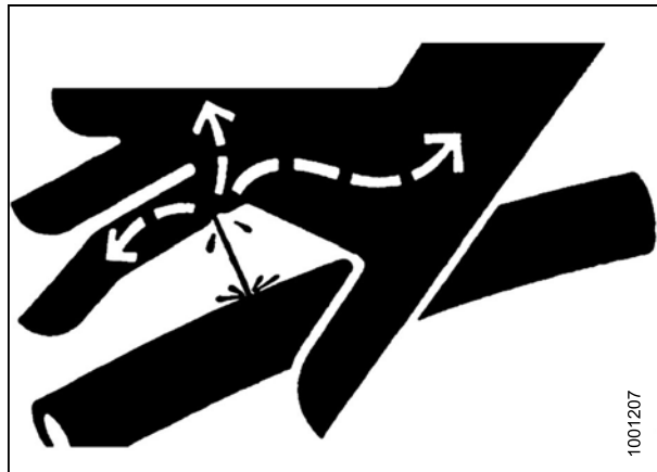
Figure 5.81: Hydraulic Pressure Hazard
