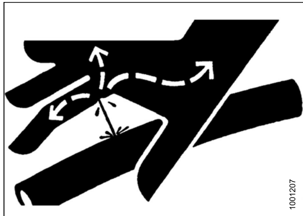
Figure 1.12: Hydraulic Pressure Hazard
