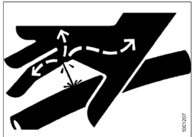
Figure 4.215: Hydraulic Pressure Hazard
