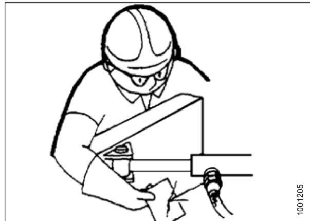
Figure 4.311: Test de fuites hydrauliques
