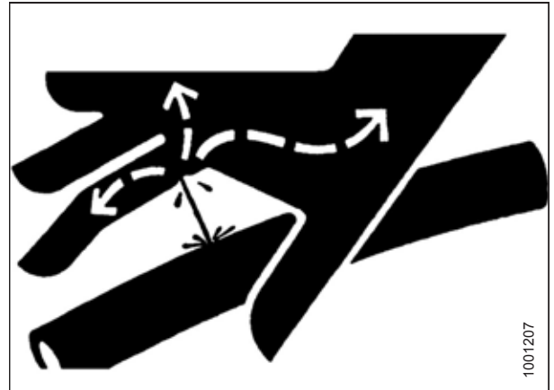
Figure 4.126: Hydraulic Pressure Hazard
