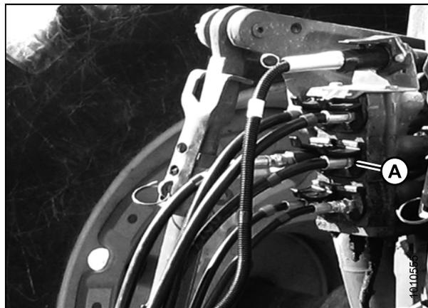
Figure 7.2: Raccord hydraulique
