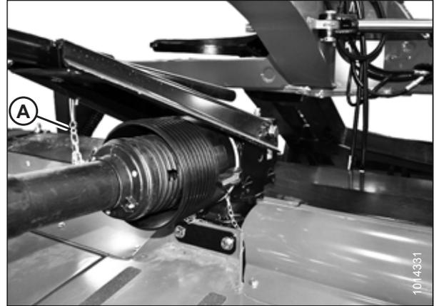
Figure 3.51: Driveline Shield
