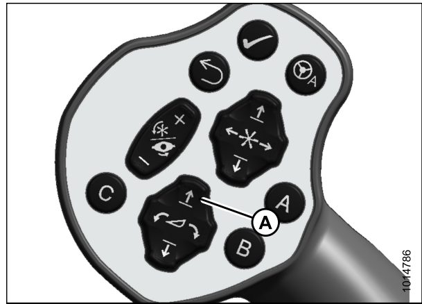
Figure 3.10: Ground Speed Lever
