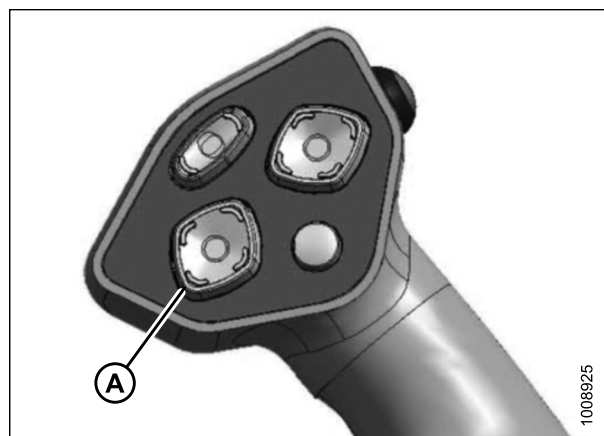
Figure 3.19: Ground Speed Lever
