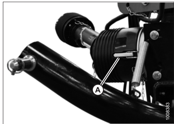
Figure 4.212: Shield Clipped to Driveline
