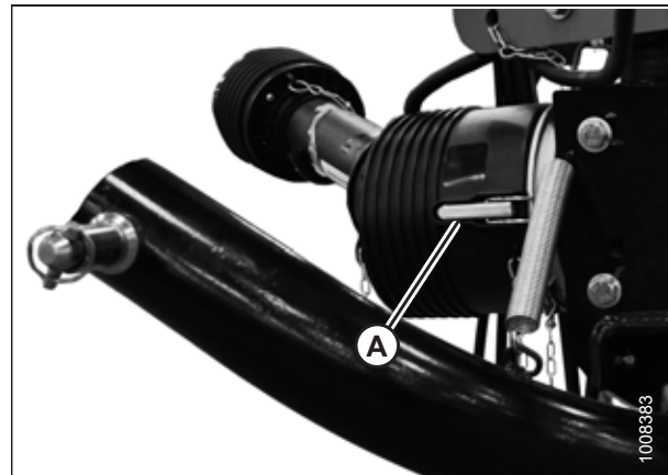
Figure 4.208: Driveline Shield Cone and Lever Clamp
