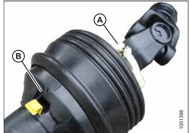
Figure 5.18: Protection de transmission
