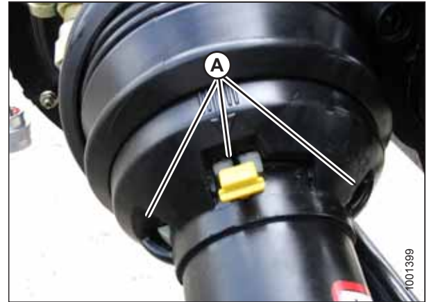
Figure 5.19: Protection de transmission
