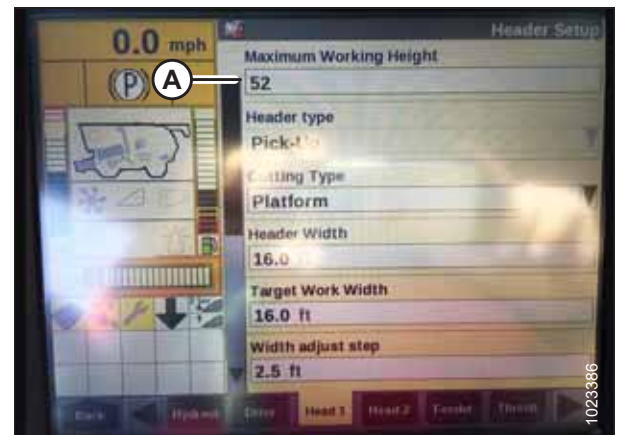
Figure 4.39: Case Combine Display – Header Setup Page
