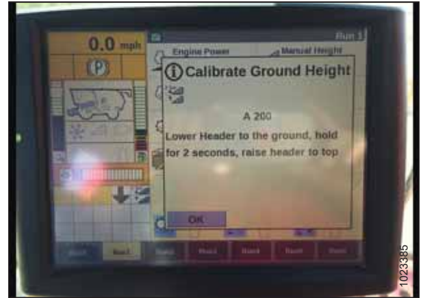
Figure 4.34: Calibrating Auto Header Height
