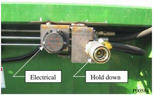
Electrical and Hydraulic Connections LH Side
