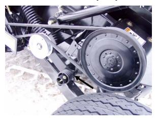
• Check that the 1/2 inch x 1 1/2 inch UNC bolt that secures the drive rotor to the large gearbox is tight. Also, check that the 1/2-inch x 1 1/2 inch UNC bolt that secures the idler rotor to the frame is tight. These bolts may work loose even though they have been drilled and secured with wire.
