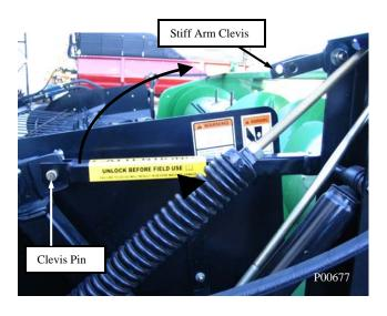
c) Place clevis pin in stiff-arm clevis and replace clip pin to secure brace upwards.
