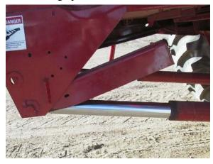
Disengaged Feeder House Lock
