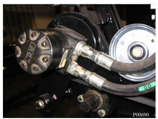
**Hydraulic Motor Installed**
