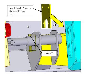
b) Guide plates are stored in the document holder on the back side of the header. Install guide plates at lower slots on standard feeder house only. Guide plates are not required with HP (Header Pitch) feeder house.
