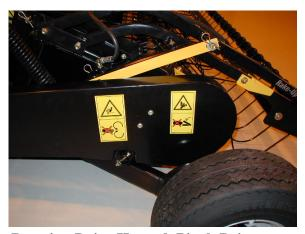
**Rotating Drive Hazard, Pinch Point Located on Belt Guard**
