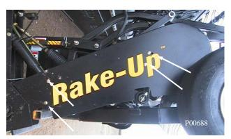
Rake-Up Drive Shield Removal
