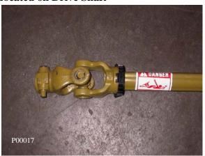
Danger, Missing Shield Located on Driveshaft (under shield)
