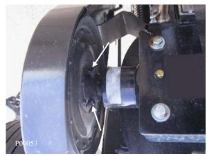
Rake-Up Main Gear Box Pulley Set Screws
