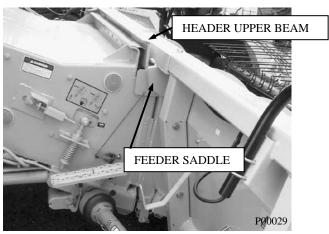
Positioning on Combine (May not be exactly as shown)
