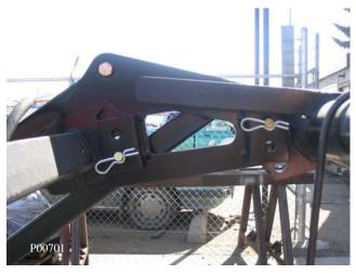
**Hold-down Clevis and Hitch Pins**
