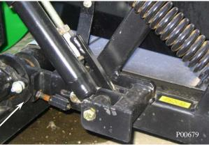
**Pickup Belt Tension Set Screws**
