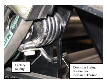
4. Tighten the tension spring hardware and put v-belt back on sheaves.
