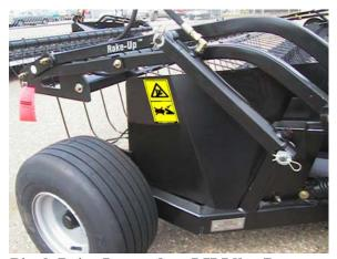
Pinch Point Located on LH Idler Rotor Shield (Rake-Up shown, SwathMaster similar)
