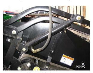
Slave Cylinder (SwathMaster pickup shown)
