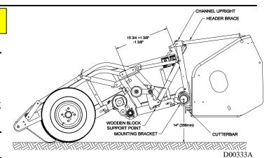
**Installing SwathMaster onto the Header**
