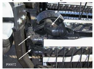
**Small Gear Box Lubrication**
