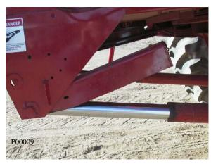
Disengaged Feeder House Lock
