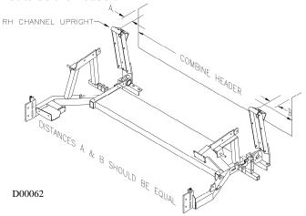
Centering the Rake-Up on the Header (Rake-Up Frame not exactly as shown)
