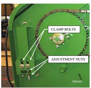
**Auger Height Adjustment Nuts**
