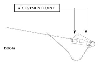
Spring Wire and Fiberglass Rod Adjustment
