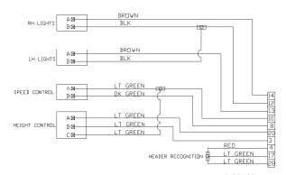
D00500 **JOHN DEERE 60 Series Wiring Harness Adapter**
