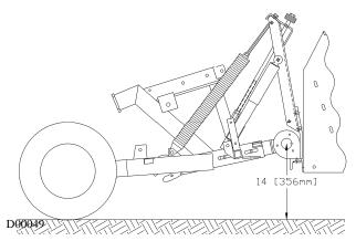
Proper Header Height (Rake-Up Shown)
