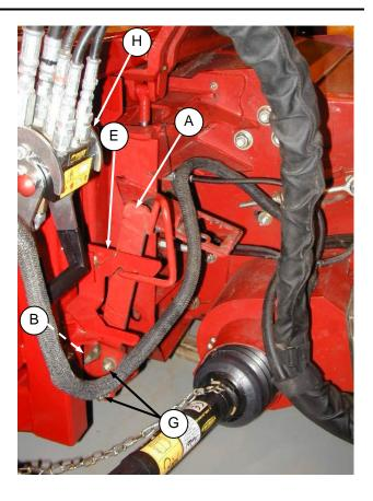
k) Disengage the feeder house locks and secure in the storage position.
