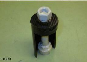
Special Tool Gearbox Puller - Part # 180784
