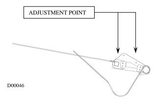
Spring Wire and Fiberglass Rod Adjustment
