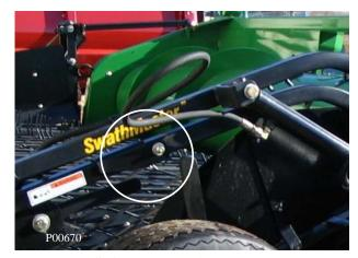
Safety Lock Disengaged
