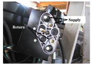
Hydraulic/Electrical Connection NOTE: When connecting/disconnecting hydraulic fittings two wrenches should be used.
