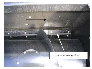
g) Attach removed stripper bar extensions to the outside of the back wall of header for storage.
