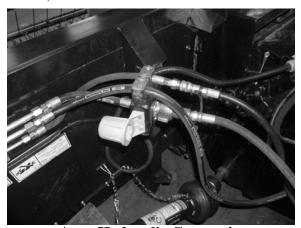
**Agco Hydraulic Connections** (Non Single Point Connector)
