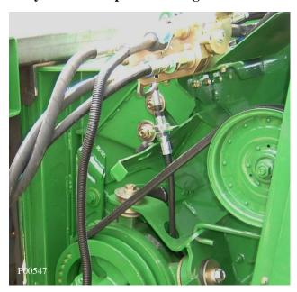
**Hydraulic Coupler in Field/Locked Position**
