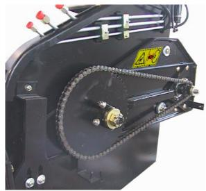
Decal, Chain Entanglement Located Above Chain (behind header LH shield)
