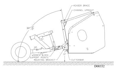
**Installing Rake-Up onto the Header**
