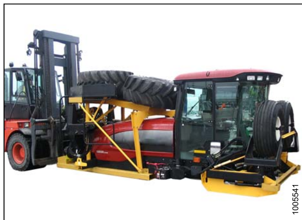
Figure 2.6: Forklift Method Lifting Points
