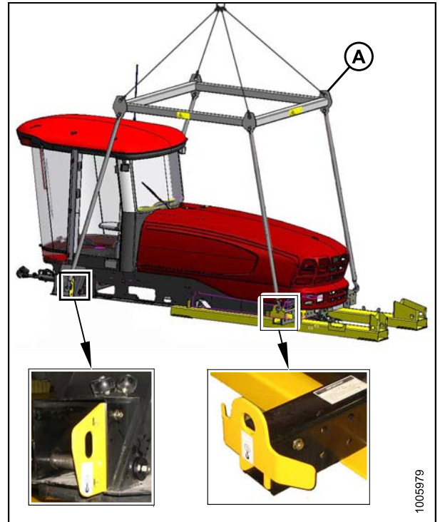
Figure 3.4: Shipping Frame Lifting Points
