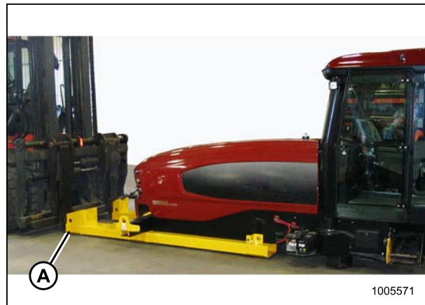
Figure 3.6: Forklift Method Lifting Points
