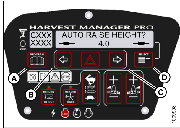
Figure 3.114: Setting Auto Raise Height
