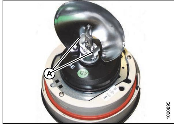
Figure 5.161: Beacon Lamp Assembly
