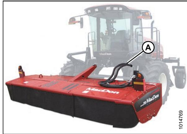
Figure 4.206: Header Connections
