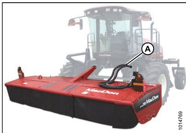
**Figure 4.214: Header Drive Hydraulics**
