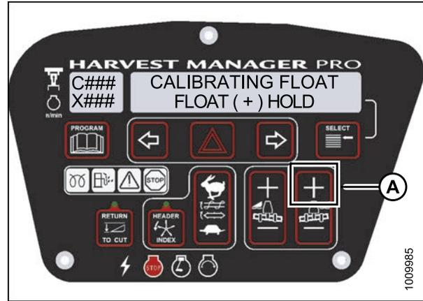
Figure 3.97: M205 Positive Header Float
