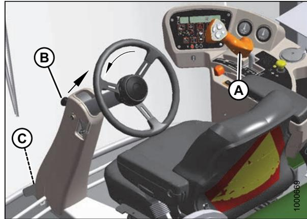
Figure 4.16: Operator Console
