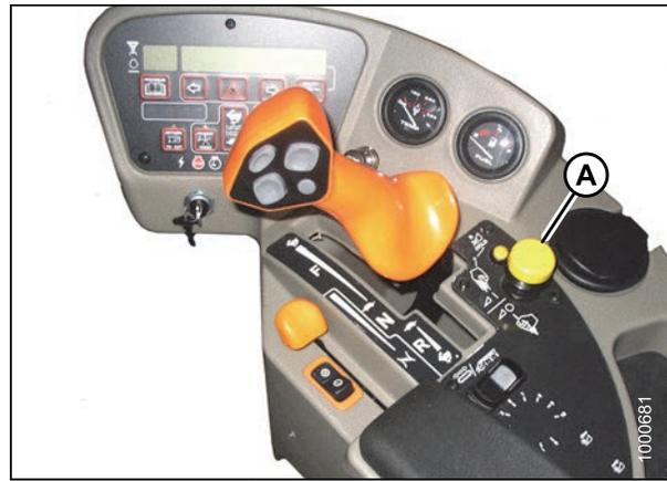
Figure 4.32: Header Drive Switch
