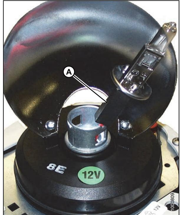
Figure 5.159: Beacon Lamp Assembly
