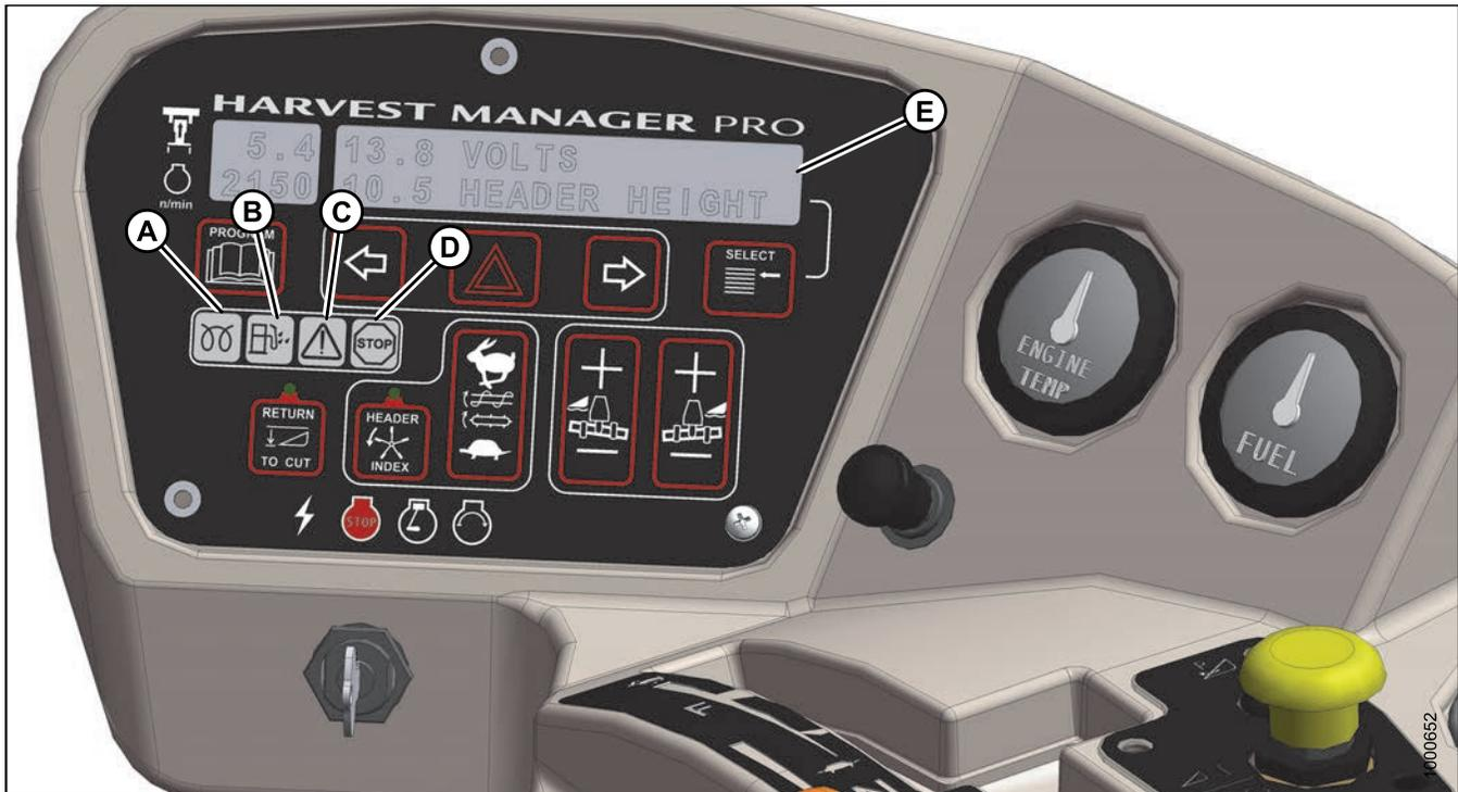
**Figure 3.69: CDM Engine Warning Lights**
