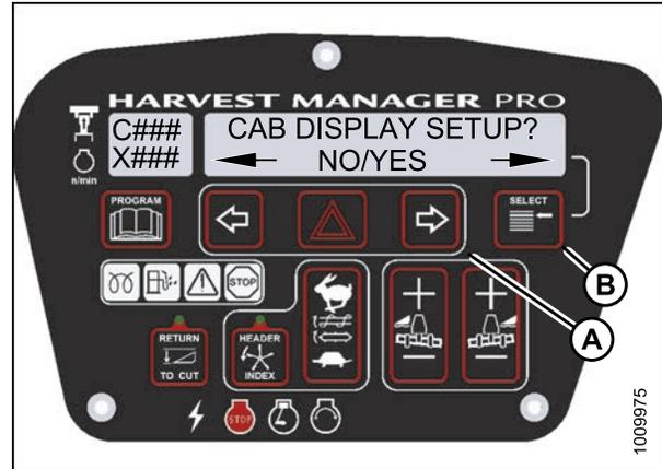
Figure 3.85: M205 Cab Display Setup
