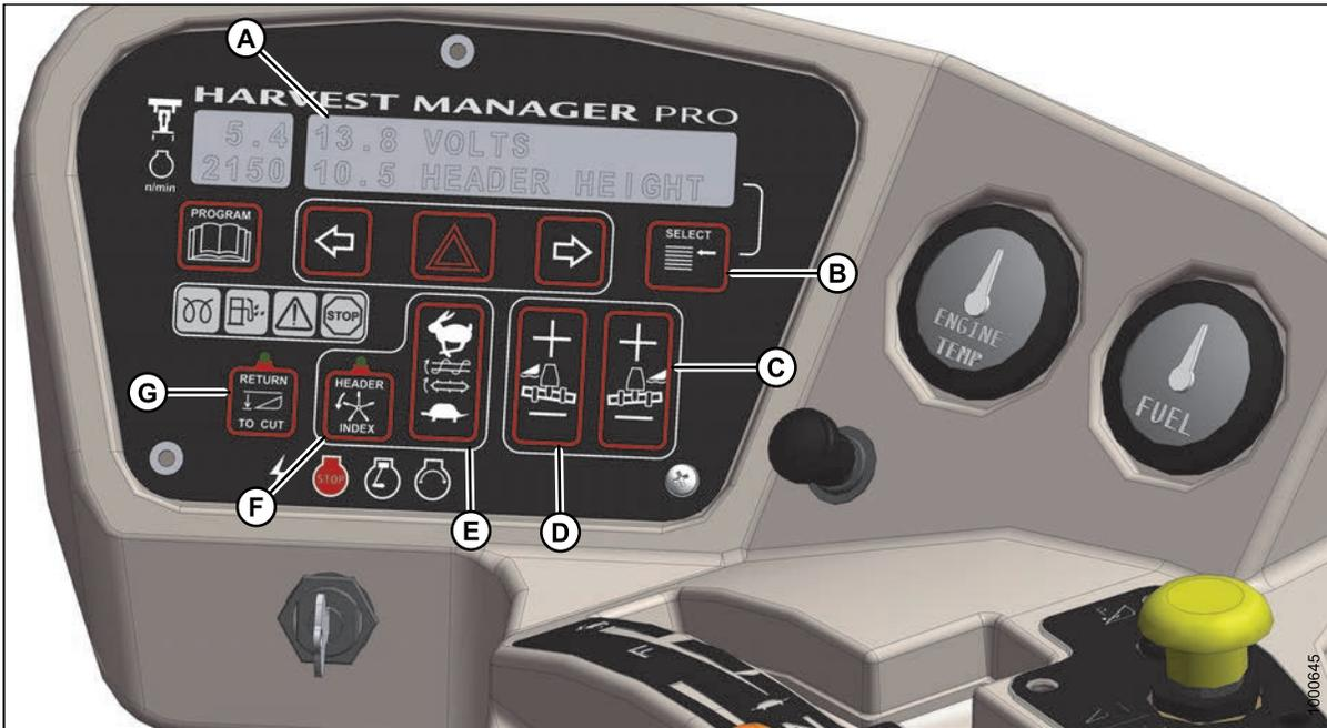
**Figure 3.67: Cab Display Module (CDM)**
