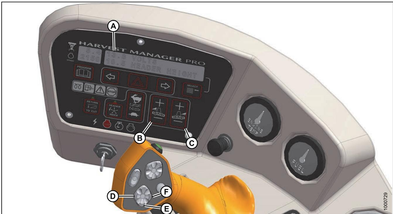
Figure 4.67: Cab Display Module (CDM) Float Adjustment
