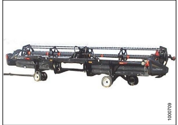
**Figure 4.39: Header in Transport Mode**
