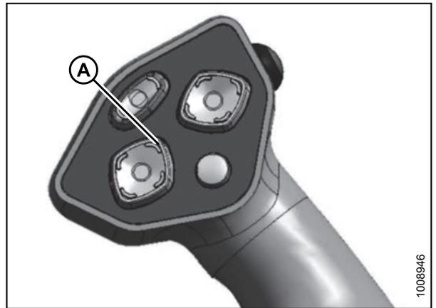
Figure 4.107: Ground Speed Lever
