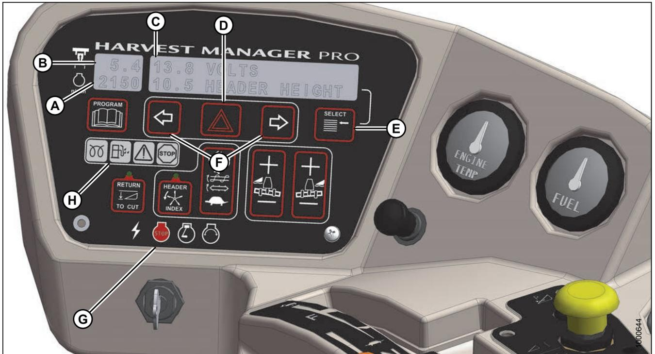
**Figure 3.66: Cab Display Module (CDM) Engine and Windrower Functions**
