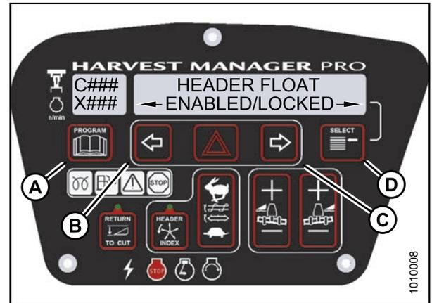
Figure 3.135: M205 Header Float Control Lock
