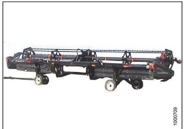
Figure 4.57: Header in Transport Mode
