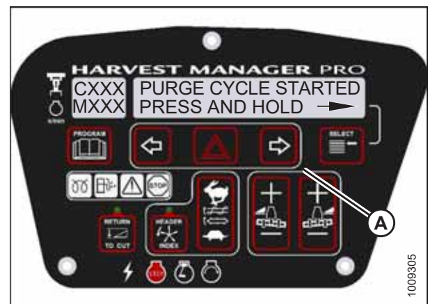
Figure 4.155: Hydraulic Purge Cycle
