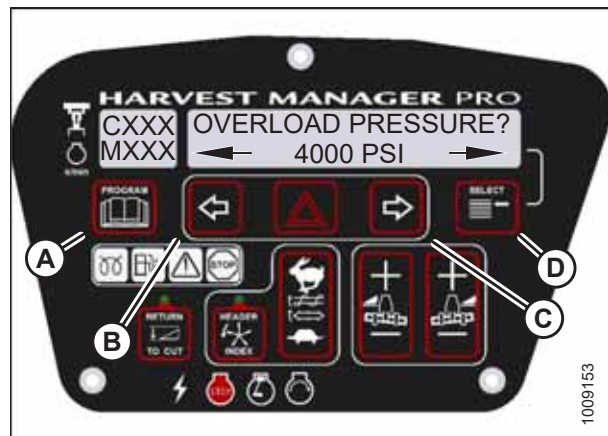
Figure 4.24: Hydraulic Overload Pressure
