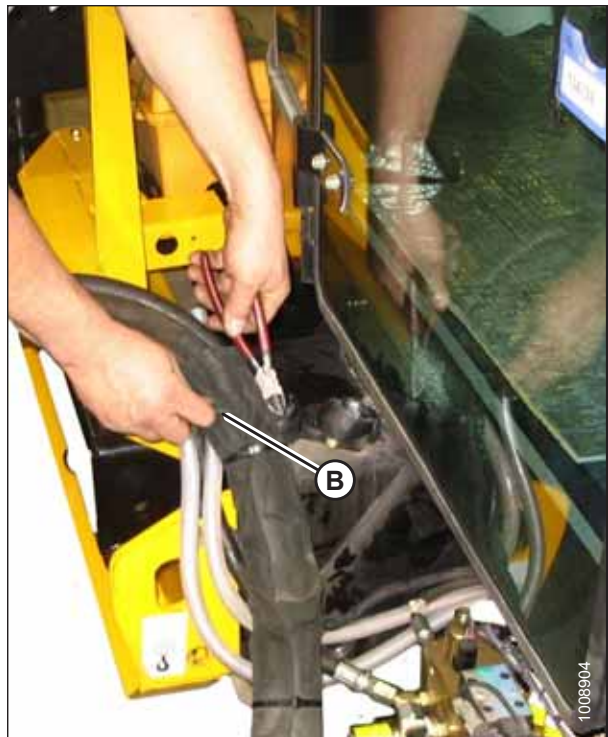
Figure 2.13: Hose Bundles on Frame
