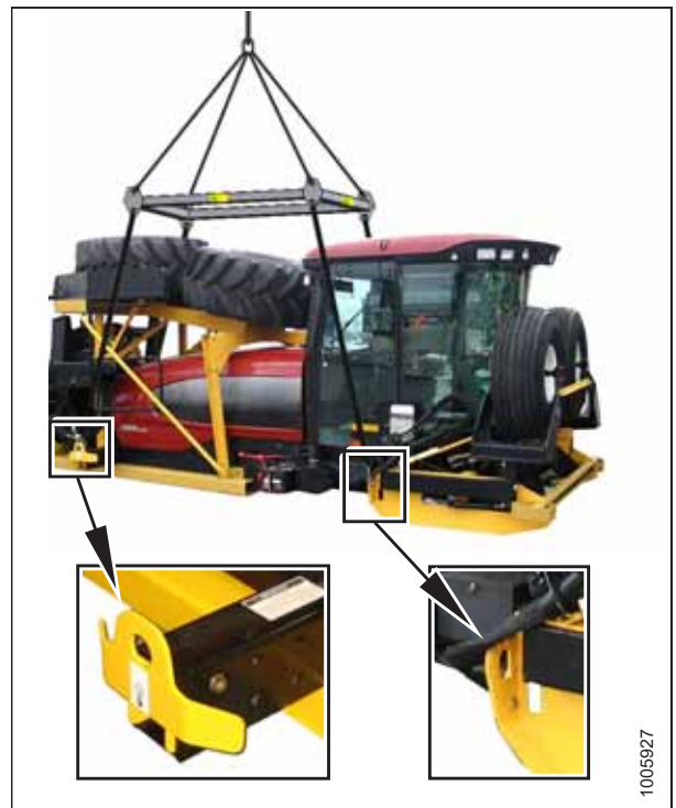
Figure 2.4: Shipping Frame Lifting Points
