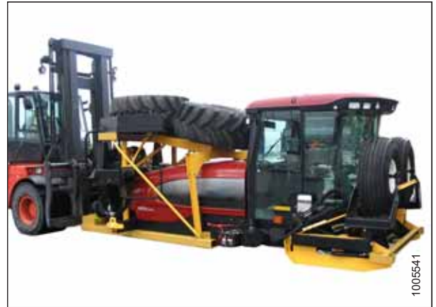
Figure 2.6: Forklift Method Lifting Points
