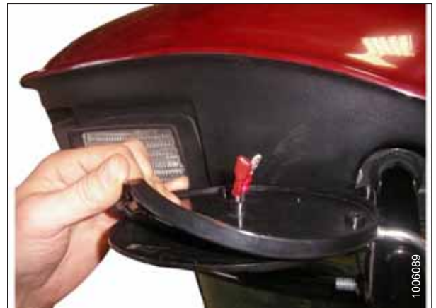
Figure 3.69: Rubber Beacon Base on Mounting Bracket
