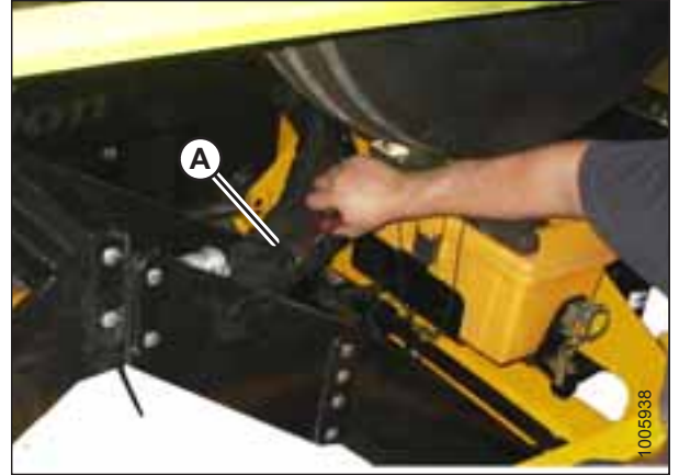
Figure 2.12: Hose Bundles on Frame
