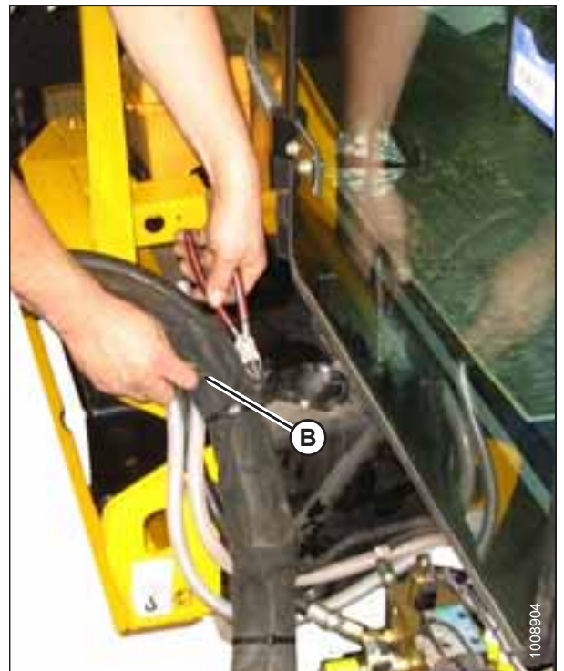
Figure 2.13: Hose Bundles on Frame
