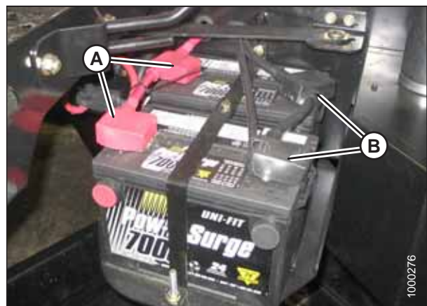
Figure 5.123: Battery Terminal Location
