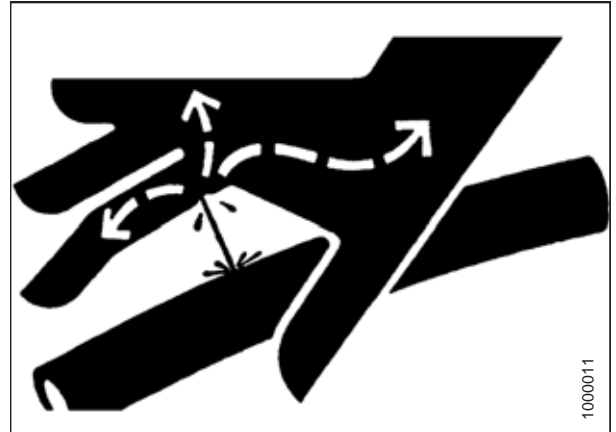
Figure 5.192: Hydraulic Pressure Hazard
