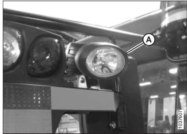
Figure 5.154: New HID Lamp in Place
