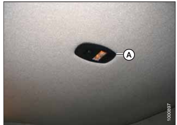
Figure 5.170: Ambient Light Fixture
