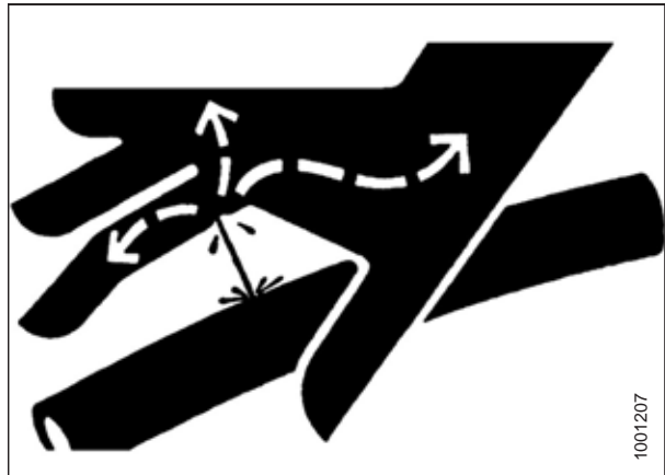
Figure 1.12: Hydraulic Pressure Hazard
