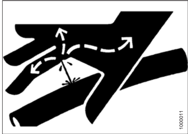
Figure 5.179: Hydraulic Pressure Hazard
