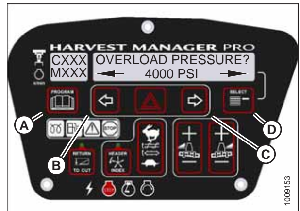
Figure 3.85: Hydraulic Overload Pressure
