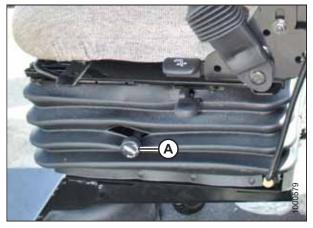
Figure 3.6: Vertical Dampener
