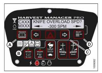
Figure 3.81: Knife Overload Speed
