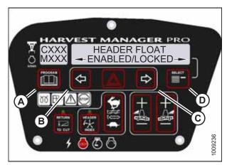
Figure 3.121: Header Float Control Lock
