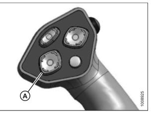
Figure 4.133: Ground Speed Lever
