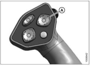
Figure 4.106: Ground Speed Lever
