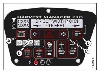
Figure 3.101: Header Cut Width
