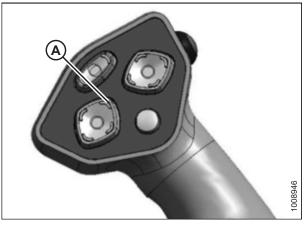
Figure 4.170: Ground Speed Lever
