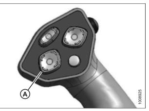
Figure 4.255: Ground Speed Lever
