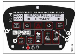
Figure 3.109: Reel Speed Display
