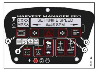
Figure 3.79: Knife Speed Setting
