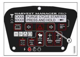
Figure 3.216: Hydraulic Purge Cycle
