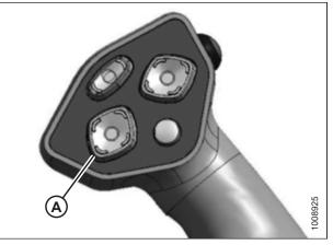
Figure 4.227: Ground Speed Lever
