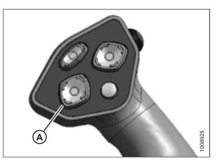
Figure 4.241: Ground Speed Lever
