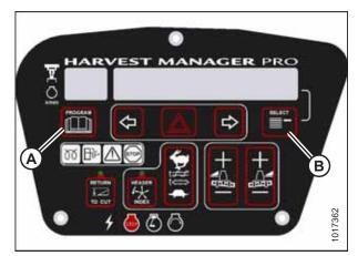
Figure 3.115: Cab Display Module (CDM)
