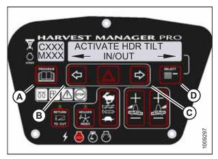
Figure 3.187: Header Tilt Angle
