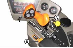
Figure 4.27: Operator Console
