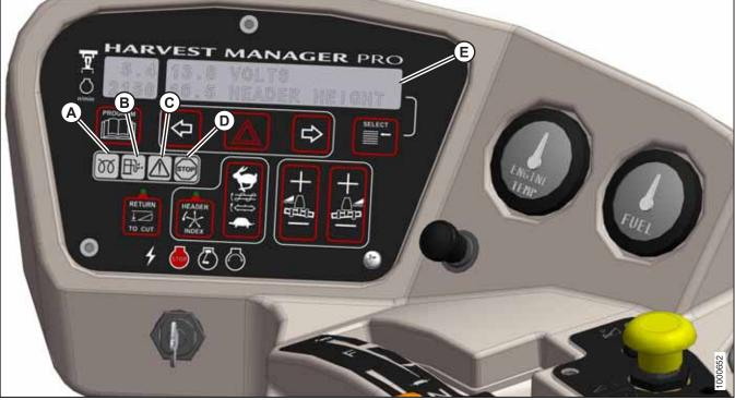
Figure 3.60: CDM Engine Warning Lights
