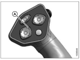
Figure 4.206: Ground Speed Lever
