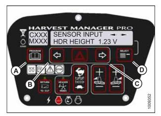
Figure 3.171: Header Sensors
