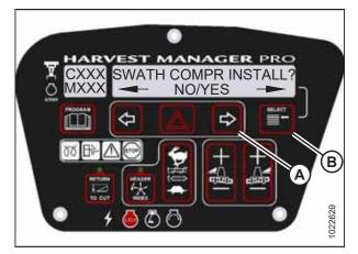
Figure 3.103: Swath Compressor Controls
