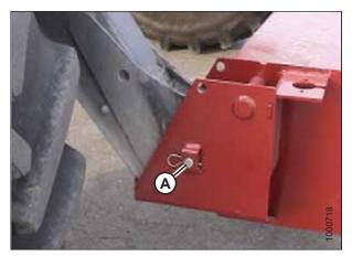
Figure 4.59: Windrower Lift Linkage
