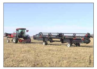
Figure 4.37: Towing a Header
