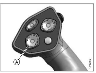
Figure 4.195: Ground Speed Lever
