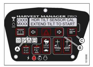
Figure 3.149: Header Tilt Calibration
