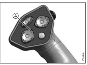
Figure 4.246: Ground Speed Lever
