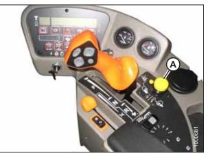
Figure 4.32: Header Drive Switch
