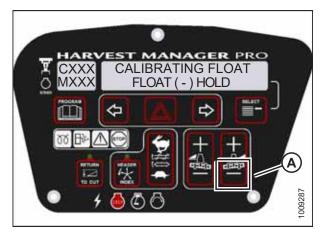
Figure 3.156: Negative Header Float Display
