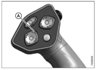
Figure 4.68: Ground Speed Lever (GSL)
