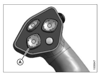
Figure 4.263: Ground Speed Lever
