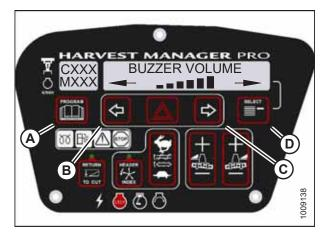
Figure 3.71: Buzzer Volume
