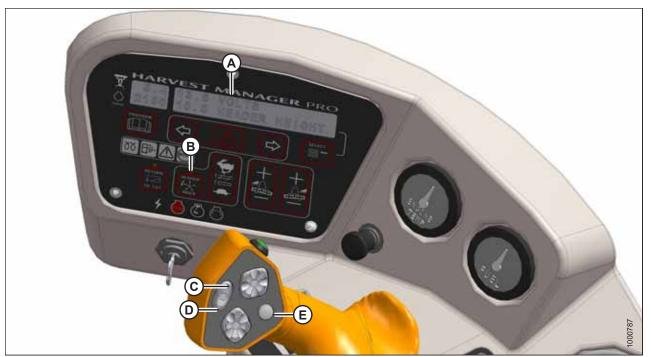
Figure 4.288: Operator Console
