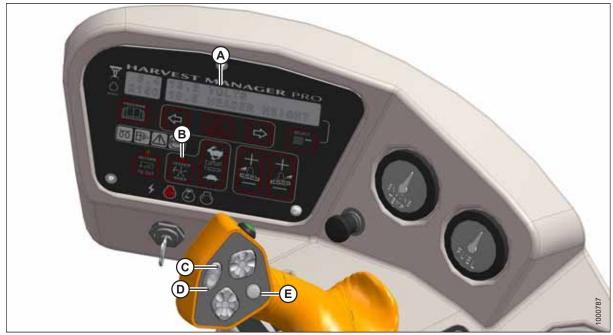
Figure 4.305: Operator Console
