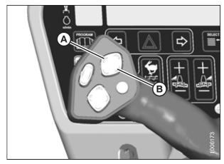
Figure 4.286: Ground Speed Lever
