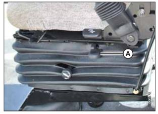
Figure 3.8: Fore-Aft Isolator Lock
