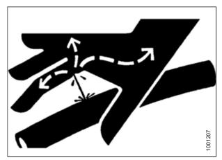
Figure 1.12: Hydraulic Pressure Hazard
