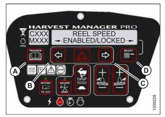
Figure 3.139: Reel Speed Control Lock
