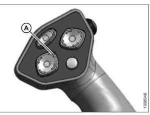
Figure 4.185: Ground Speed Lever
