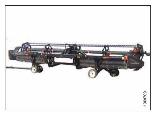
Figure 4.40: Header in Transport Mode
