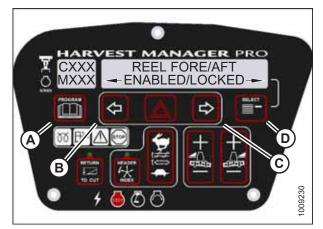
Figure 3.124: M155 Reel Fore-Aft Control Lock
