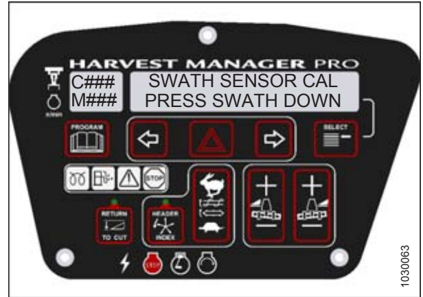
Figure 3.156: Swath Compressor Sensor Calibration
