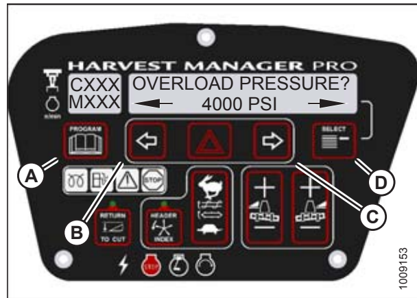
Figure 3.85: Hydraulic Overload Pressure
