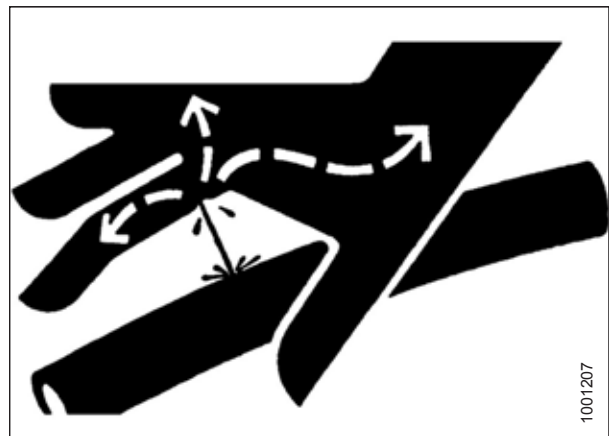
Figure 1.12: Hydraulic Pressure Hazard
