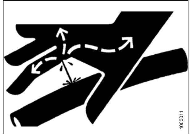
Figure 5.188: Hydraulic Pressure Hazard
