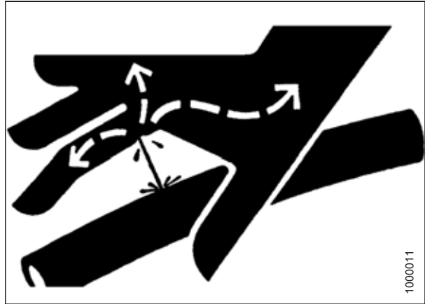
Figure 5.175: Hydraulic Pressure Hazard
