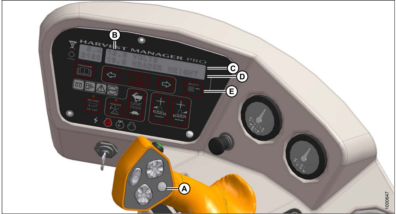
Figure 3.58: CDM Operating Screen
