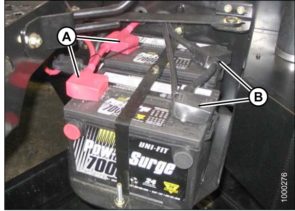
Figure 5.121: Battery Terminal Location
