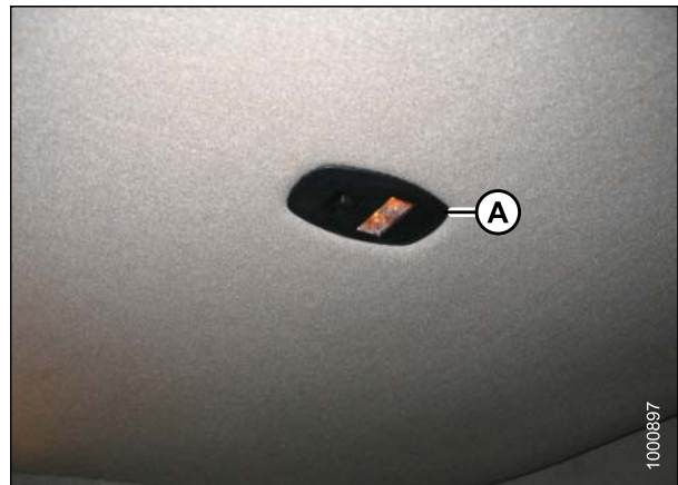
Figure 5.167: Ambient Light Fixture
