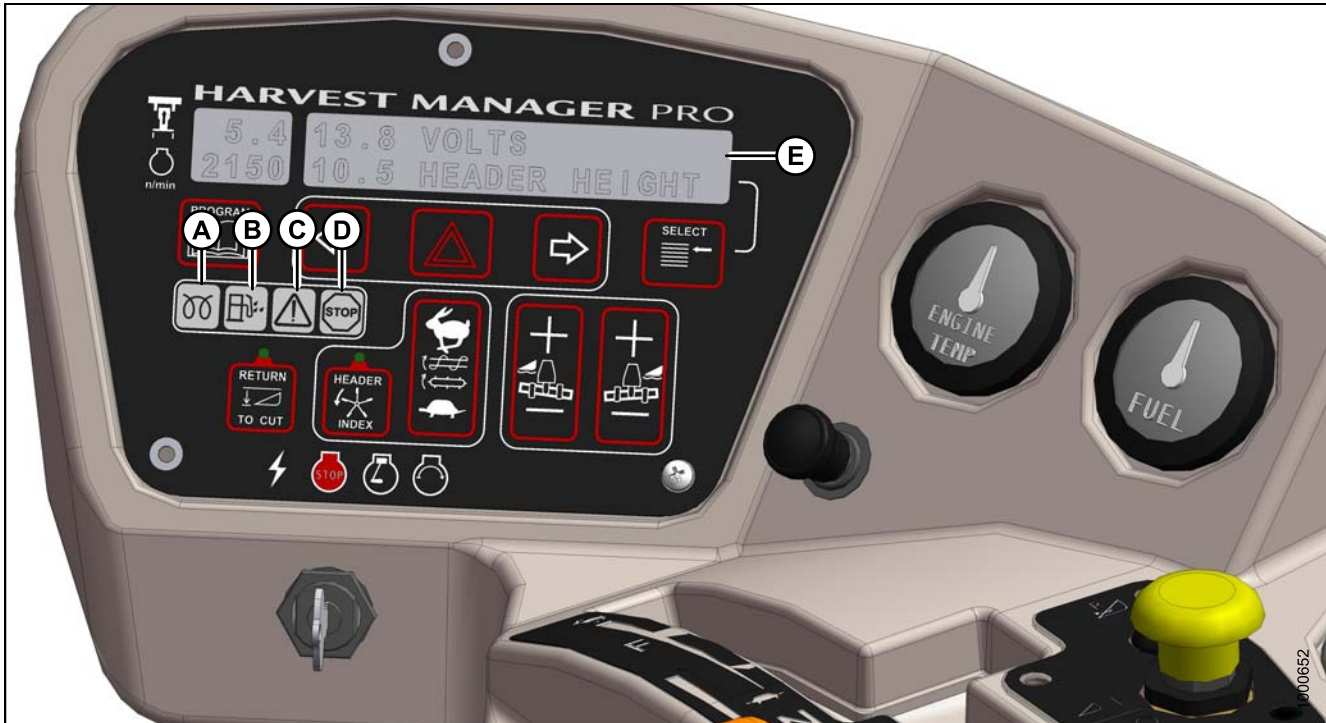
Figure 3.59: CDM Engine Warning Lights
