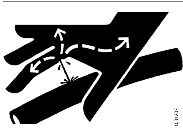
Figure 1.12: Hydraulic Pressure Hazard
