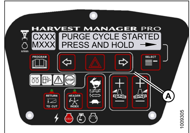
Figure 3.208: M155 Hydraulic Purge Cycle
