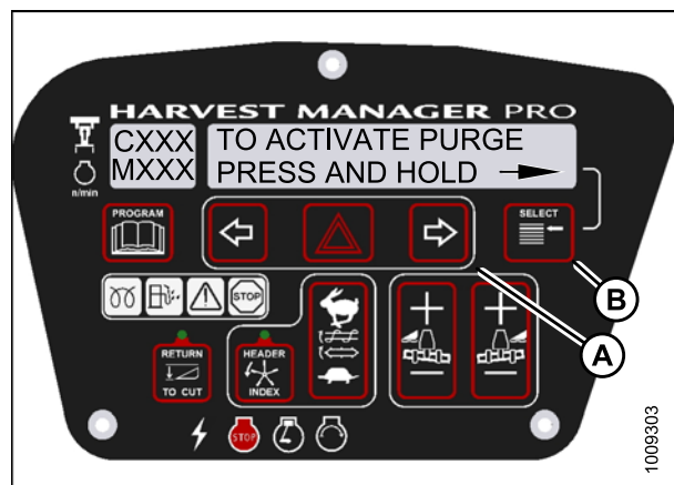
Figure 3.207: M155 Hydraulic Purge
