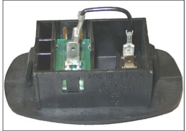
Figure 5.168: Ambient Light Fixture
