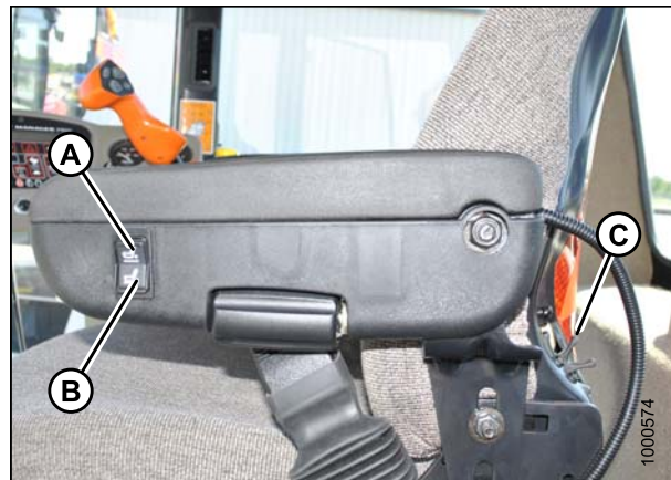
Figure 3.5: Seat Suspension and Height
