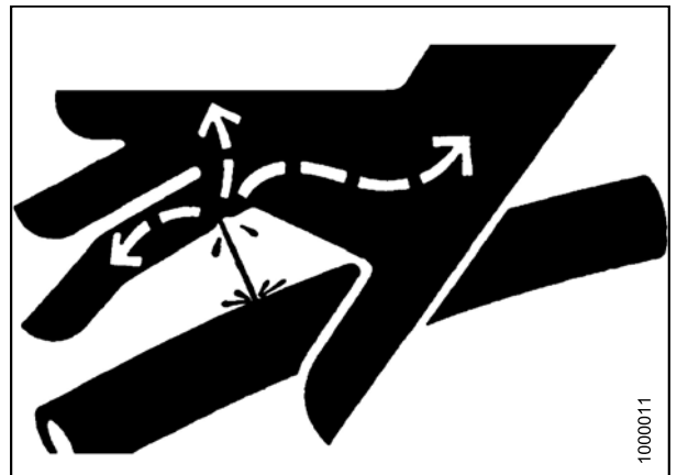
Figure 5.207: Hydraulic Pressure Hazard
