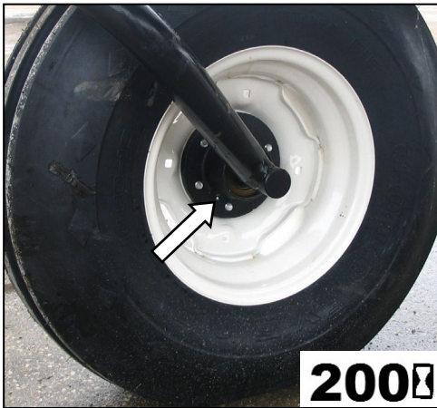
FORMED CASTER WHEEL BEARING 1 PLACE (BOTH WHEELS)
